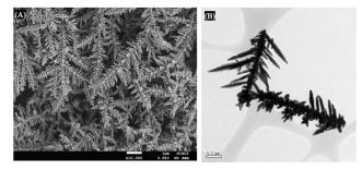
(A) SEM and (B) TEM images of Ir/Au-D after 20-hour stability
