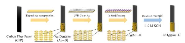
Fig. 1 Schematic illustration of the fabrication process for three-dimensional dendritic gold (Au-D), Ir/Au-D, and IrO<sub>2</sub>/Au-D catalysts.
