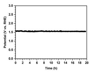
Fig. 8 Chronopotentiometric stability test of Ir/Au-D in 1.0 M KOH at a constant current density of 10 mA cm<sup>-2</sup>.
