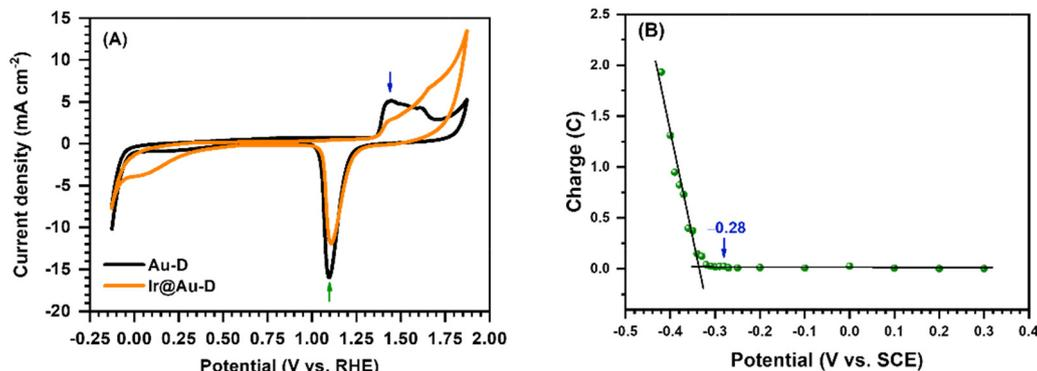
Fig. 2 (A) Cyclic voltammograms (CVs) of Au-D (black line) and Ir@Au-D (orange line) recorded in 0.5 M H<sub>2</sub>SO<sub>4</sub> at a scan rate of 10 mV s<sup>-1</sup>. (B) Plot of charge versus potential during Cu underpotential deposition (UPD); the applied potential is referenced to the SCE electrode used in the actual experiment.
