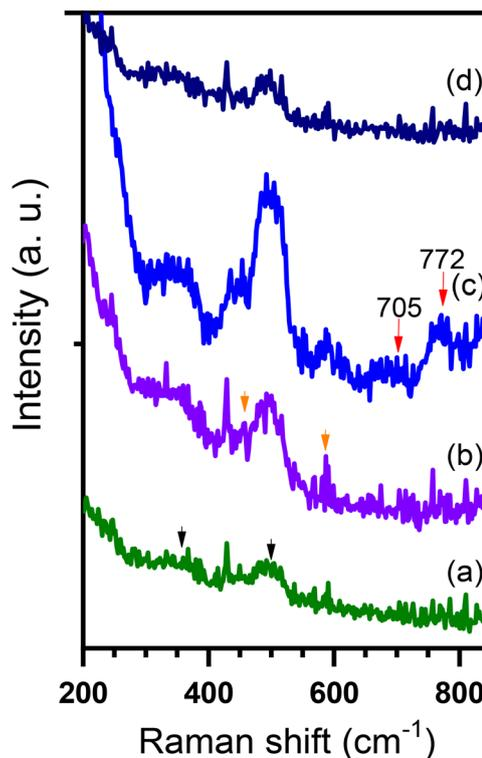
Fig. 10 *In situ* SERS spectra of Ir/Au-D during OER: (a) at open circuit potential (OCP), (b) at  $-0.27 \text{ V}$ , (c) at  $-0.30 \text{ V}$ , and (d) after the reaction (OCP). The spectrum for each potential condition represents the average of 20 scans.
