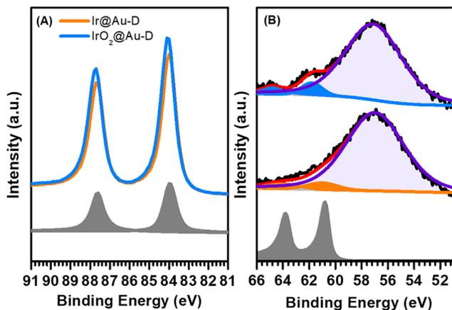
Fig. 6 X-ray photoelectron spectroscopy (XPS) analysis: (A) Au 4f spectra of Au-D (gray), Ir/Au-D (orange), and IrO<sub>2</sub>/Au-D (blue). (B) Ir 4f and Au 5p spectra of Ir wire (gray), Ir/Au-D (orange), and IrO<sub>2</sub>/Au-D (blue).
