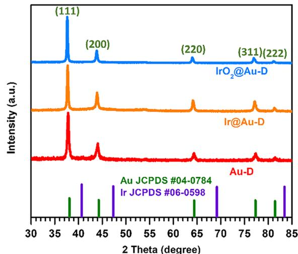
Fig. 5 X-ray diffraction (XRD) patterns of Au-D, Ir/Au-D, and IrO<sub>2</sub>/Au-D. Reference diffraction data are based on Au (JCPDS #04-0784) and Ir (JCPDS #06-0598).
