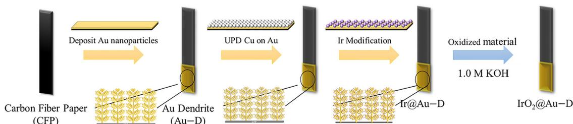
Fig. 1 Schematic illustration of the fabrication process for three-dimensional dendritic gold (Au-D), Ir/Au-D, and IrO<sub>2</sub>/Au-D catalysts.
