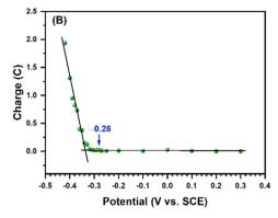
Fig. 2 (A) Cyclic voltammograms (CVs) of Au-D (black line) and Ir/Au-D (orange line) recorded in  $0.5 \text{ M} \text{ H}_2\text{SO}_4$  at a scan rate of 10 mV s<sup>-1</sup>. (B) Plot of charge *versus* potential during Cu underpotential deposition (UPD); the applied potential is referenced to the SCE electrode used in the actual experiment.
