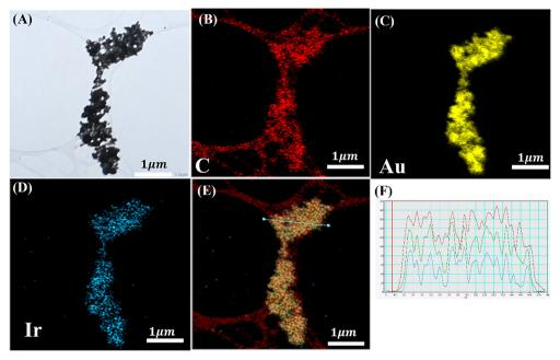
Fig. 4 Transmission electron microscopy (TEM) and energy-dispersive X-ray spectroscopy (EDS) analysis of Ir/Au-D detached from the CFP electrode. (A) TEM image of Ir/Au-D. (B) – (D) EDS elemental maps showing the distribution of (B) carbon (C), (C) gold (Au), and (D) iridium (Ir). (E) Overlay of EDS maps illustrating the spatial distribution of C, Au, and Ir. (F) EDS line-scan profile of Ir/Au-D form(E), with red representing C, green for Au, and blue for Ir.
