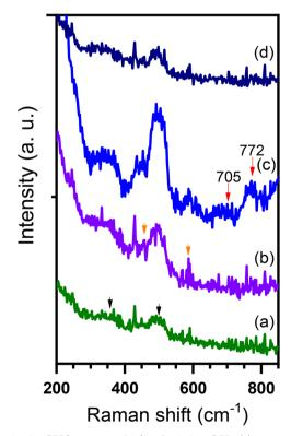
Fig. 10 In situ SERS spectra of Ir/Au-D during OER: (a) at open circuit potential (OCP), (b) at -0.27 V, (c) at -0.30 V, and (d) after the reaction (OCP). The spectrum for each potential condition represents the average of 20 scans.
