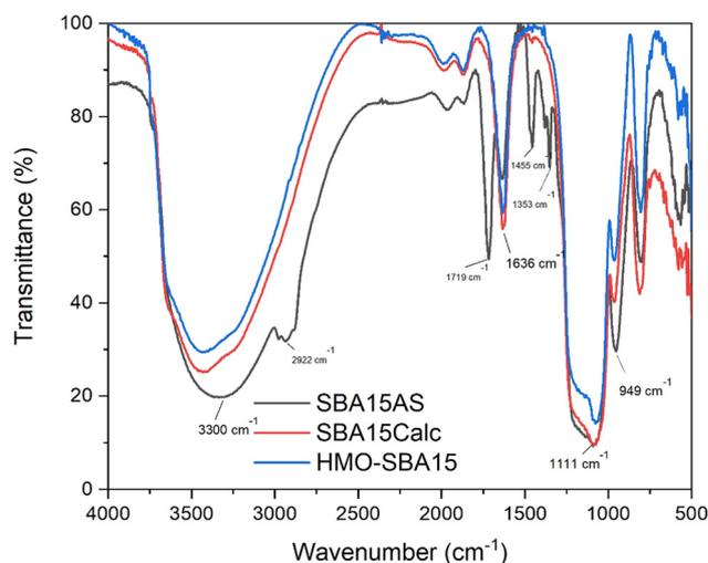
Fig. 4 FTIR spectral overlap of samples AS, calc and HMO.
