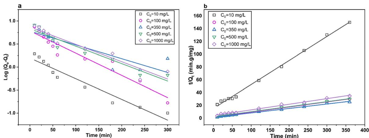
Fig. 6 (a) Pseudo-first and (b) second order models of the adsorption kinetics.
