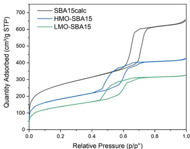
Fig. 3 Nitrogen adsorption-desorption isotherms of samples SBA15<sub>calc</sub>, HMO-SBA15 and LMO-SBA15.
