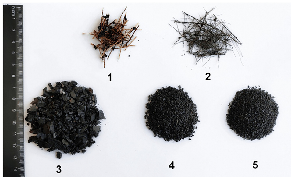
Fig. 2 Typical products of cryogrinding. 1 – nylon cord, 2 – metal cord, 3 – large size fraction of rubber crumb (1–5 mm), 4 – mean size fraction (1–2 mm), 5 – small size fraction (0.1–1 mm). Reproduced from ref. 7.
