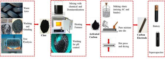
Fig. 11 The process of waste tire conversion into energy device. Reproduced from ref. 44.
