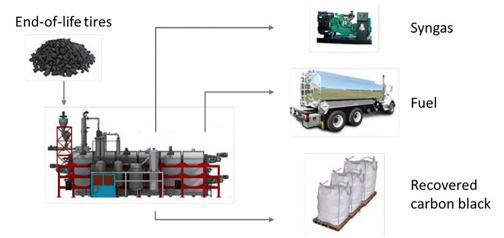
Fig. 3 Schematic representation of ELT pyrolysis and ensuing products. Reproduced from ref. 23.
