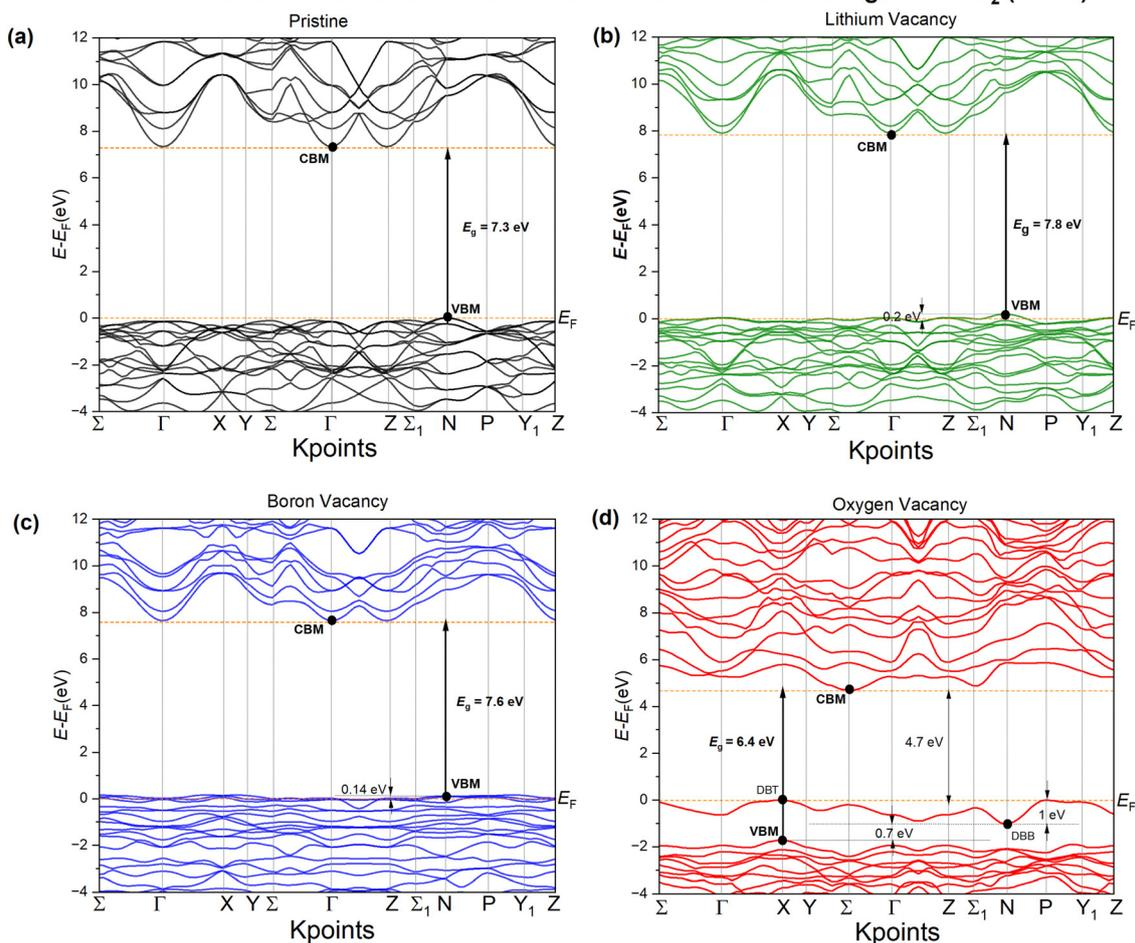
Fig. 2 Calculated electronic band structure of tetragonal LiBO<sub>2</sub> (t-LBO) for (a) pristine, (b) Li-vacancy, (c) B-vacancy, and (d) O-vacancy supercells. The conduction band minimum, valence band maximum, defect band top, and defect band bottom are abbreviated as CBM, VBM, DBT, and DBB, respectively.
