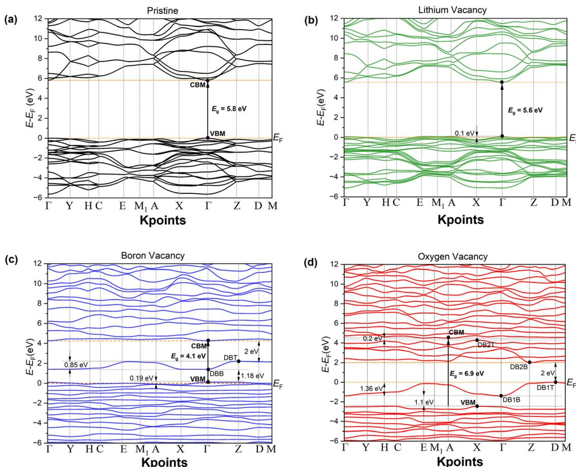
Fig. 3 Calculated electronic band structure of monoclinic LiBO<sub>2</sub> (m-LBO) for (a) pristine, (b) Li-vacancy, (c) B-vacancy, and (d) O-vacancy supercells. The conduction band minimum, valence band maximum, defect band 1 top, defect band 1 bottom, defect band 2 top, and defect band 2 bottom are abbreviated as CBM, VBM, DB1T, DB1B, DB2T, and DB2B, respectively.
