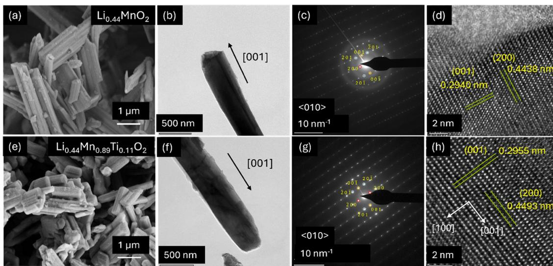
Fig. 3 Morphology analysis. (a) and (e) SEM images of  $\text{Li}_{0.44}\text{MnO}_2$  (LMO1) and  $\text{Li}_{0.44}\text{Mn}_{0.89}\text{Ti}_{0.11}\text{O}_2$  (LMO2). (b), (c) and (d) TEM image, SAED pattern and HRTEM image of LMO1. (f), (g) and (h) TEM image, SAED pattern and HRTEM image of LMO2. The  $\langle 010 \rangle$  zone axis was taken for the SAED patterns.
