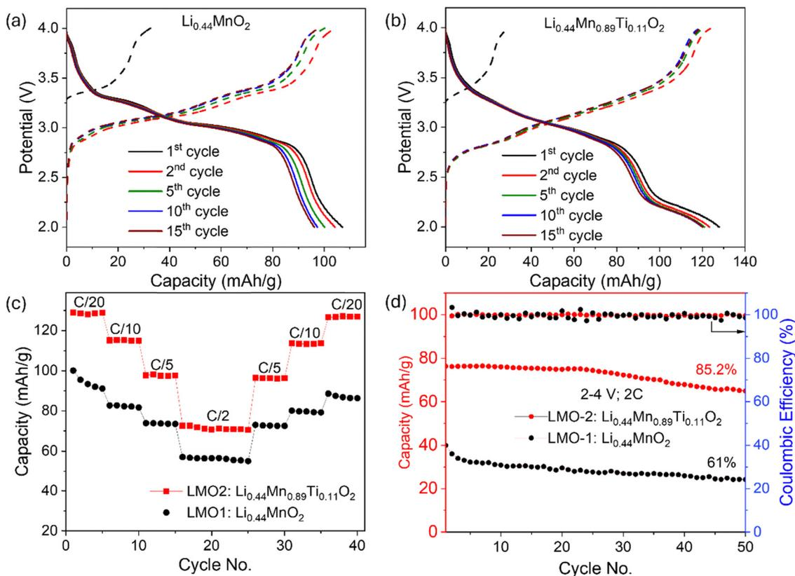
Fig. 4 Galvanostatic charge/discharge profiles for (a) pristine  $\text{Li}_{0.44}\text{MnO}_2$  (LMO1) and (b) Ti-doped  $\text{Li}_{0.44}\text{Mn}_{0.89}\text{Ti}_{0.11}\text{O}_2$  (LMO2) compositions cycled at a rate of C/20 (2–4 V). (c) Corresponding rate kinetics for LMO1 and LMO2. (d) Cycling stability and coulombic efficiency of LMO1 and LMO2 cycled at a fast rate of 2C in the voltage window of 2–4 V.
