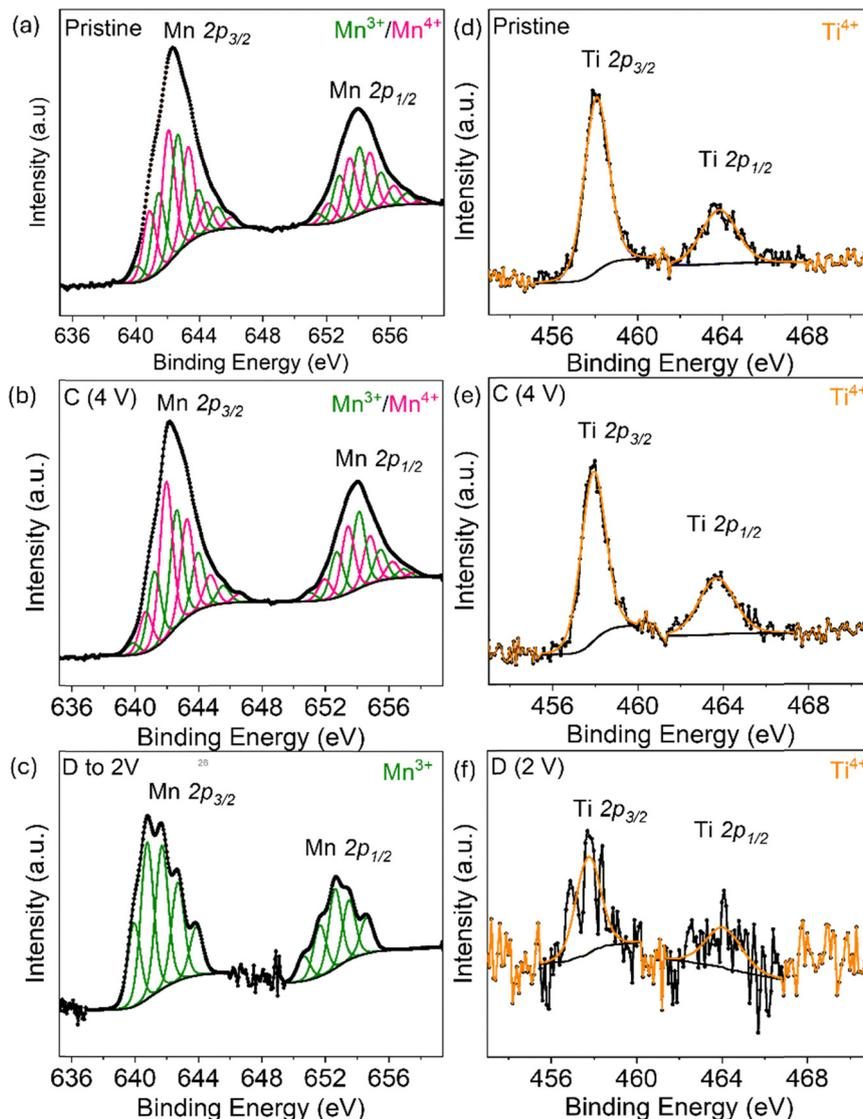
Fig. 5 Mn 2p XPS spectra of LMO2: (a) pristine cathode, (b) cathode charged to 4 V, and (c) cathode discharged to 2 V. Mn<sup>4+</sup>/Mn<sup>3+</sup> redox states are captured. Ti 2p XPS spectra of LMO2: (d) pristine state, (e) charged to 4 V, and (f) discharged to 2 V. The Ti<sup>4+</sup> redox state remain unaltered.
