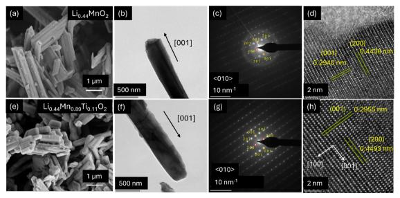
Fig. 3 Morphology analysis. (a) and (e) SEM images of  $Li_{0.44}$ MnO<sub>2</sub> (LMO1) and  $Li_{0.44}$ MnO<sub>8.9</sub>Ti<sub>0.11</sub>O<sub>2</sub> (LMO2). (b), (c) and (d) TEM image, SAED pattern and HRTEM image of LMO2. The  $\langle 010 \rangle$  zone axis was taken for the SAED patterns.
