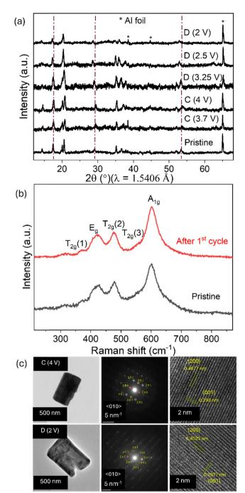
Fig. 6 (a) Ex situ XRD patterns of LMO2 at different states of charge. (b) Comparative Raman spectra of LMO2 in pristine and after the 1st cycle. (c) Ex situ TEM, SAED and HRTEM analysis of the LMO2 cathode charged to 4 V (top) and discharged to 2 V (bottom). The  $\langle 010 \rangle$  zone axis was taken for the SAED patterns.
