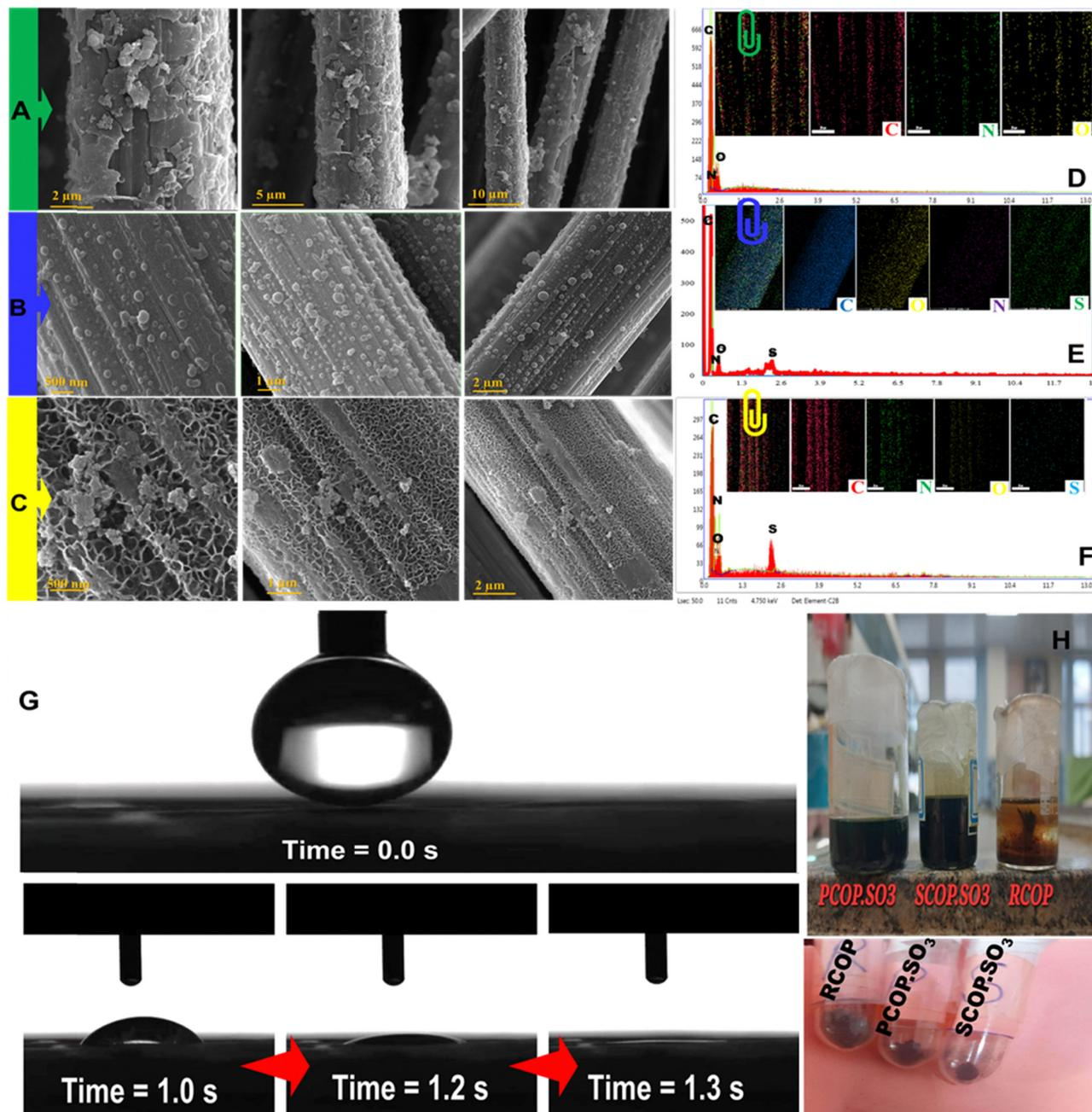
**Fig. 1** FE-SEM images and the corresponding elemental mapping images of the (A) FCF@RCOP, (B) FCF@SCOP-SO<sub>3</sub> and (C) FCF@PCOP-SO<sub>3</sub>. (D)–(F) are the equivalents EDXA and mapping analyses from (A) to (C) respectively. (G) The time-lapse of the contact angle experiment undertaken on FCF@PCOP-SO<sub>3</sub>. (H) The dried synthesized COPs collected from the bottom of the beaker and the corresponding solution prior to filtration and drying.
