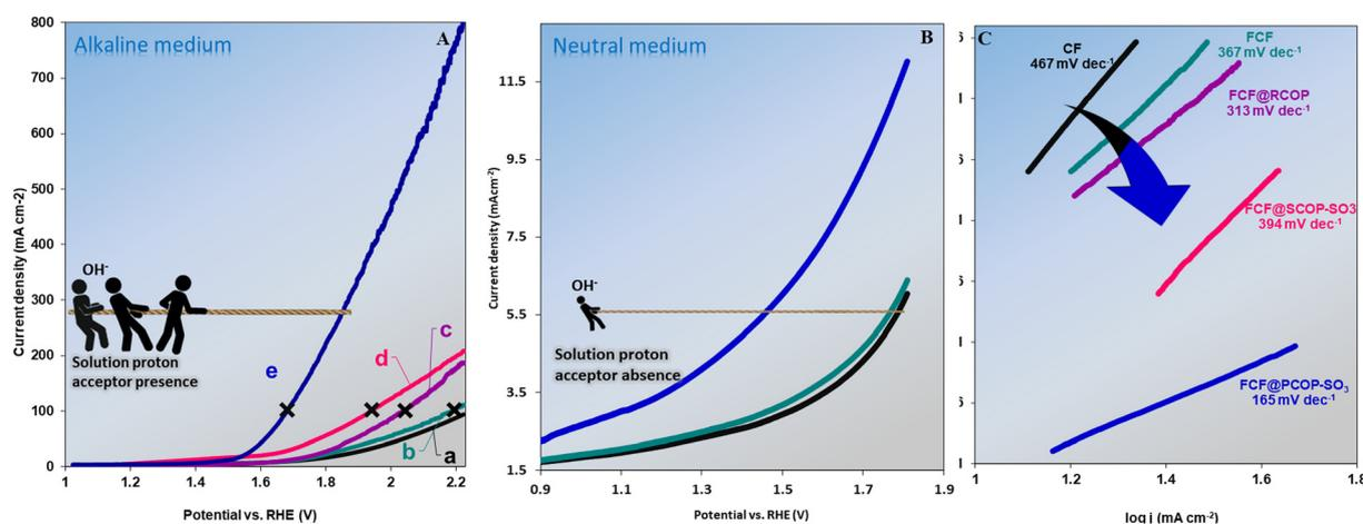
Fig. 4 (A) and (B) LSVs recorded in 0.1 M of KOH and phosphate buffer (pH=7), respectively, with a sweep rate of 5 mVs<sup>-1</sup> at (a) CF, (b) FCF, (c) FCF@RCOP, (d) FCF@SCOP-SO<sub>3</sub> and (e) FCF@PCOP-SO<sub>3</sub>. (C) The corresponding Tafel plot for CF (blue), FCF (brown), FCF@RCOP (green), FCF@SCOP-SO<sub>3</sub> (violet) and FCF@PCOP-SO<sub>3</sub> (red).
