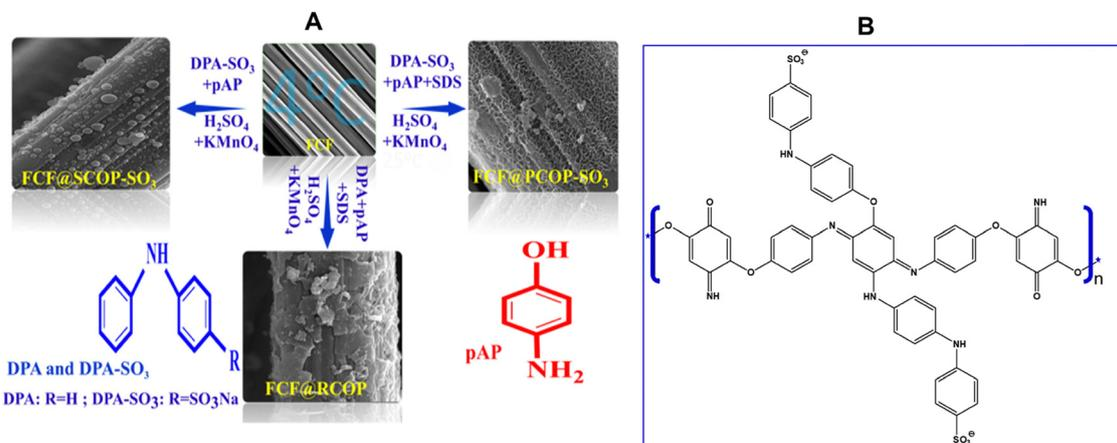
**Scheme 1** (A) Synthesis and schematic illustration of FCF@RCOP, FCF@SCOP-SO<sub>3</sub>, and FCF@PCOP-SO<sub>3</sub> from *p*-aminophenol, and substituted diphenylamine at 4 °C. (B) The proposed profile of the synthesized polymer including DPA-SO<sub>3</sub> + pAP.
