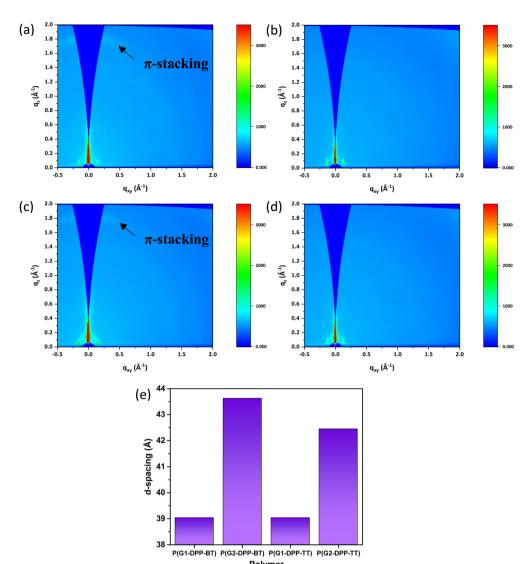
Fig. 4 Solid-state nanostructure in thin films investigated using X-ray scattering. Grazing incidence wide-angle X-ray scattering (GIWAXS) 2D patterns of (a) P(G1-DPP-BT), (b) P(G2-DPP-BT), (c) P(G1-DPP-TT), and (d) P(G2-DPP-TT) and (e) lamellar spacing of P(G1-DPP-BT), P(G2-DPP-BT), P(G1-DPP-TT), and P(G2-DPP-TT), extracted from GIWAXS 2D patterns.
