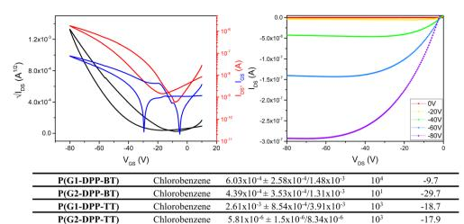
\*Device mobilities, ON/OFF ratios and threshold voltages have been averaged from a minimum of 10 or more devices for each polymer. Each device was fabricated from the same batch for each polymer.
