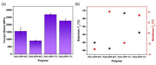
Fig. 5 Thermomechanical properties of the semiconducting polymers with poly(benzyl ether) dendrons. (a) Young's moduli of P(G1-DPP-BT), P(G2-DPP-BT), P(G1-DPP-TT), and P(G2-DPP-TT) from quantitative nanomechanical mapping (AFM) and (b) backbone (red) and side chain (black) glass transition temperatures  $(T_0)$  determined through dynamic mechanical analysis (DMA).
