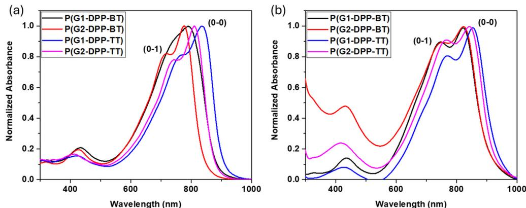
Fig. 2 Optical properties of the semiconducting polymers with poly(benzyl ether) side chains. UV-Vis spectra of **P(G1-DPP-BT)**, **P(G2-DPP-BT)**, **P(G1-DPP-TT)**, and **P(G2-DPP-TT)** in (a) solution in  $\text{CHCl}_3$  and (b) thin film after thermal annealing at  $150^\circ\text{C}$  for 1 hour.
