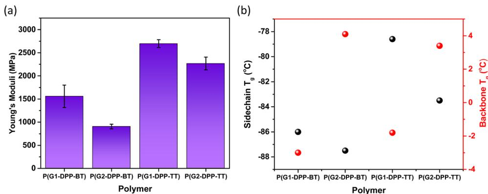
Fig. 5 Thermomechanical properties of the semiconducting polymers with poly(benzyl ether) dendrons. (a) Young's moduli of **P(G1-DPP-BT)**, **P(G2-DPP-BT)**, **P(G1-DPP-TT)**, and **P(G2-DPP-TT)** from quantitative nanomechanical mapping (AFM) and (b) backbone (red) and side chain (black) glass transition temperatures ( $T_g$ ) determined through dynamic mechanical analysis (DMA).
