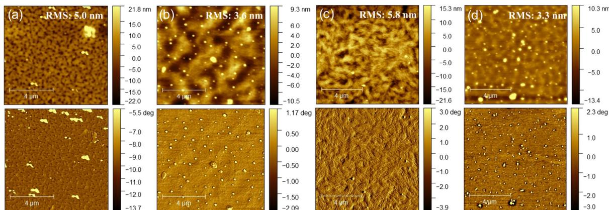
Fig. 3 Nanoscale morphology of the semiconducting polymers with poly(benzyl ether) dendrons. Atomic force microscopy (AFM) (a) height (top) and phase (bottom) images of **P(G1-DPP-BT)**; (b) height (top) and phase (bottom) images of **P(G2-DPP-BT)**, (c) height (top) and phase (bottom) images of **P(G1-DPP-TT)** and (d) height (top) and phase (bottom) images of **P(G2-DPP-TT)** after thermal annealing at  $150^\circ\text{C}$  for 1 hour. The scale bar is  $4\ \mu\text{m}$ .
