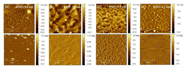
Fig. 3 Nanoscale morphology of the semiconducting polymers with poly(benzyl ether) dendrons. Atomic force microscopy (AFM) (a) height (top) and phase (bottom) images of **P(G1-DPP-BT)**, (b) height (top) and phase (bottom) images of **P(G2-DPP-BT)**, (c) height (top) and phase (bottom) images of **P(G1-DPP-TT)** after thermal annealing at 150 °C for 1 hour. The scale bar is 4  $\mu$ m.
