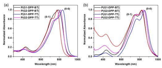
Fig. 2 Optical properties of the semiconducting polymers with poly(benzyl ether) side chains. UV-Vis spectra of **P(G1-DPP-BT)**, **P(G2-DPP-BT)**, **P(G1-DPP-TT)**, and **P(G2-DPP-TT)** in (a) solution in CHCl<sub>3</sub> and (b) thin film after thermal annealing at 150 °C for 1 hour.
