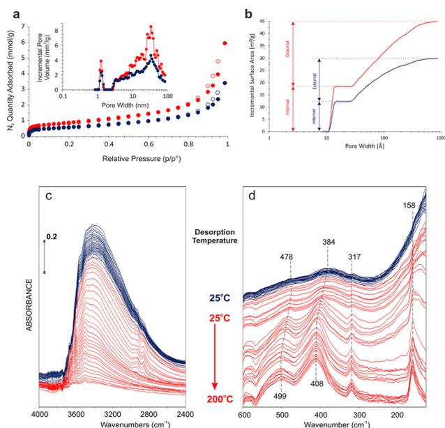
**Fig. 2** (a) Low-temperature N<sub>2</sub> adsorption (inset: pore size distribution), (b): cumulative surface area distribution, (c) and (d): the FTIR spectra registered during the temperature-programmed desorption (note that blue and red colors are for nW-CuO(25) and nW-CuO(200), respectively).
