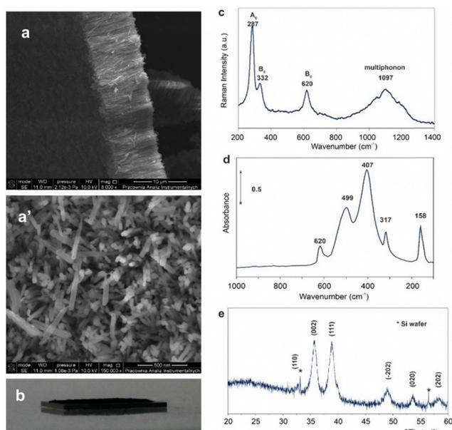
**Fig. 1** (a) and (a'): SEM pictures of synthesized nanowires nW-CuO, and its (b): water contact angle (WCA) equal to zero. Structural characterization: (c): Raman; (d): far IR; (e): XRD (note that only the FIR sample was vacuum treated at 200 °C).
