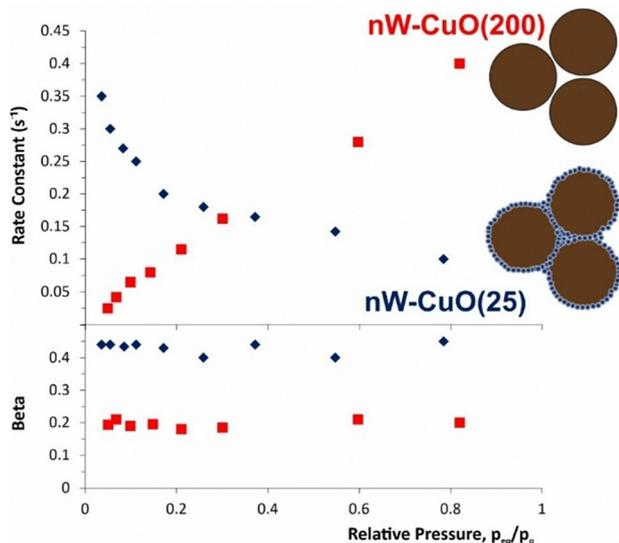
Fig. 5 Changes in the rate constant and  $\beta$ -parameter during  $\text{H}_2\text{O}$  adsorption on nW-CuO(200) – red and nW-CuO(25) – blue.
