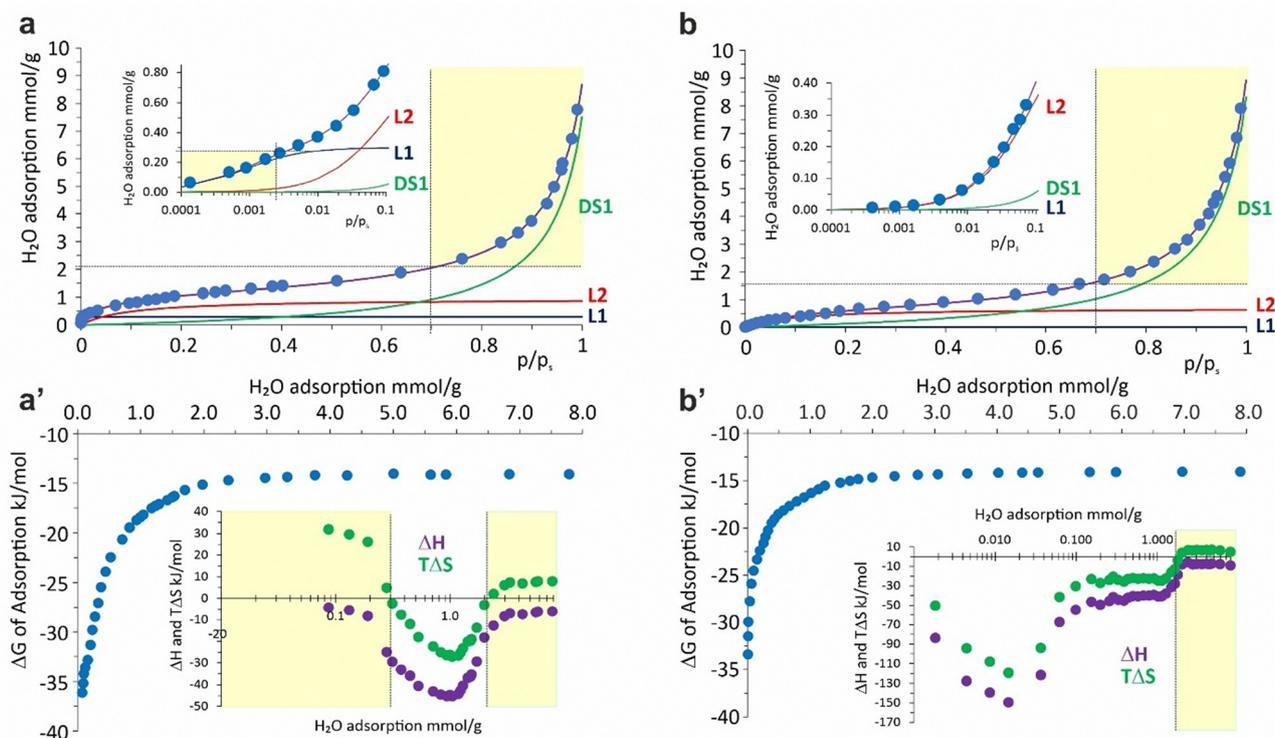
**Fig. 4** Water adsorption isotherm on (a): nW-CuO(200) (b): nW-CuO(25). Marked areas are for entropy-derived Gibbs free energy changes, which are shown in (a') and (b'); note that insets in (a') and (b') show changes in the values of the components of the  $\Delta G$ .
