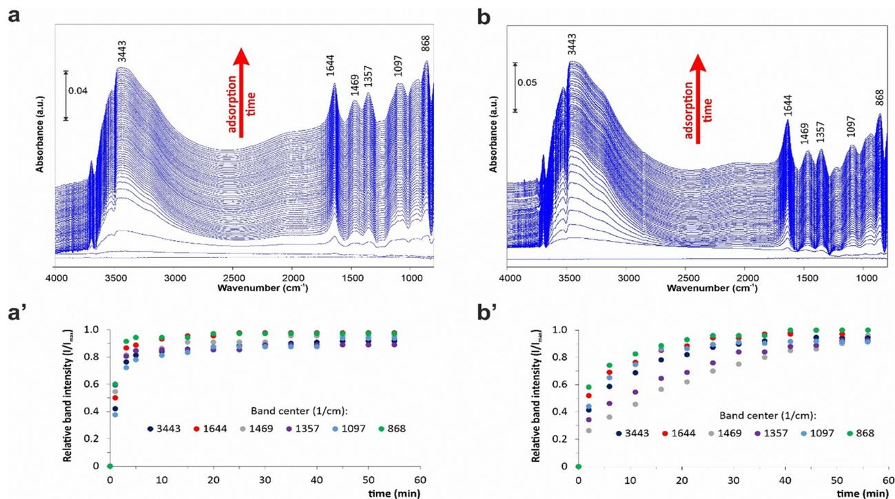
Fig. 6 Spectral changes induced by  $\text{H}_2\text{O}$  adsorption on (a) nW-CuO(200) and (b) nW-CuO(25). The bottom panels (a') and (b') collect the quantitative data (note that  $p/p_s = 0.9$ , in Ar with a total flow rate of  $50 \text{ mL min}^{-1}$  was used).
