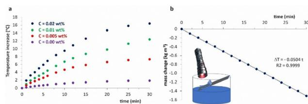
**Fig. 3** (a) Temperature changes of the solutions under irradiation with an 805 nm laser (0.8 W cm<sup>-2</sup>) and (b) the corresponding solar-to-vapor generation efficiency during evaporation under an equivalent of 0.5 sun.
