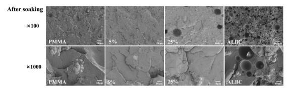
Fig. 6 SEM images at 100× and 1000× magnifications of PMMA bone cement, 5% and 25% FUMA bone cement, and ALBC after soaking
