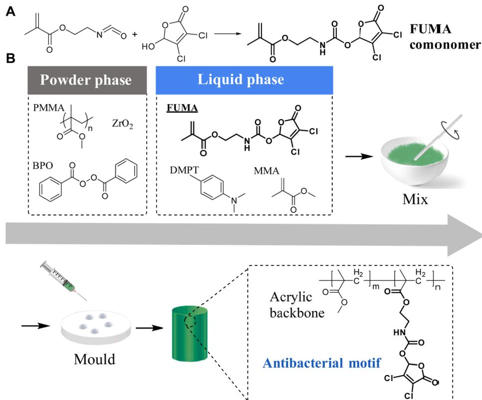
**Fig. 1** (A) Synthetic route of FUMA (see Section 2.2 for details); (B) the FUMA cement was fabricated by mixing the solid phase with the liquid phase containing FUMA. The mixture was stirred until it reached the dough phase, then filled into the mold. After curing, the cement was removed from the mold.
