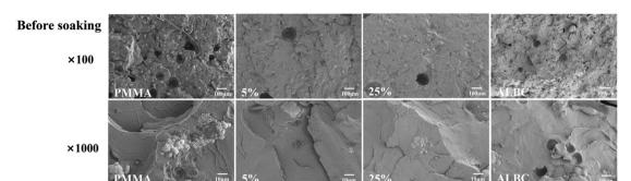
SEM images at 100× and 1000× magnifications of PMMA bone cement, 5% and 25% FUMA bone cement, and ALBC before soaking
