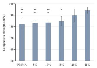
**Fig. 3** Compressive strength of PMMA bone cement and FUMA bone cements (\*. p < 0.05, indicates a significant difference compared to 25% FUMA bone cement, \*\*. p < 0.01, indicates a highly significant difference. ^. p < 0.05, indicates a significant difference compared to 20% FUMA bone cement).
