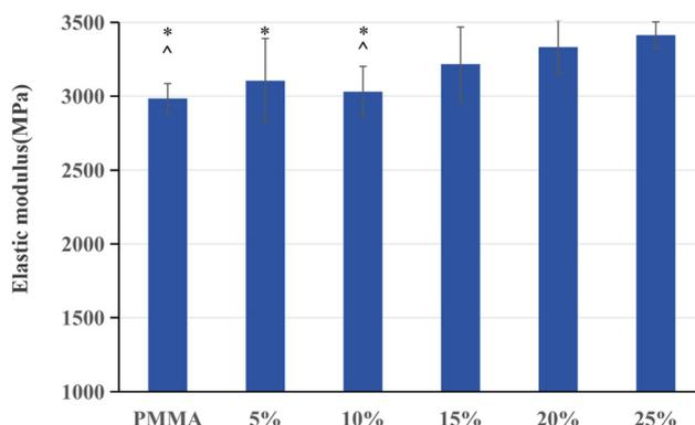
Fig. 4 Elastic modulus of PMMA bone cement and FUMA bone cements (\*.  $p < 0.05$ , indicates a significant difference compared to 25% FUMA bone cement, ^.  $p < 0.05$ , indicates a significant difference compared to 20% FUMA bone cement).
