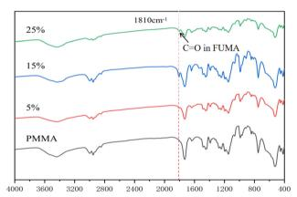
Fig. 2 FT-IR spectra of PMMA bone cement and FUMA bone cements.
