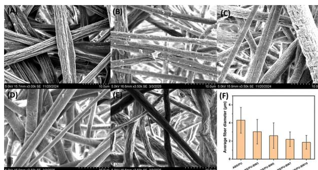
Fig. 1 SEM images of the electrospun ABS/PU samples at different beeswax concentrations. (A) ABS/PU, (B) ABS/PU–BW3, (C) ABS/PU–BW5, (D) ABS/PU–BW7, (E) ABS/PU–BW10, and (F) average fibre diameter of the ABS/PU samples at different beeswax concentrations.
