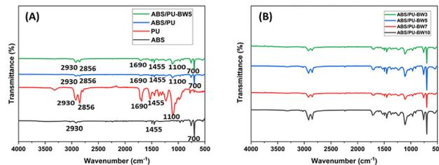
Fig. 3 IR spectra of (A) ABS, PU, ABS/PU and ABS/PU-BW5, and (B) IR spectra, and increment of the C-H stretching peak with the increase in beeswax concentration.
