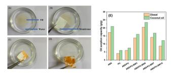
Fig. 8 (A)-(D) Images of selective absorption of diesel from the water surface with ABS/PU-BW5 membranes. (E) Maximum oil absorption capacity of various concentrations of ABS/PU-BW membranes in diesel and
