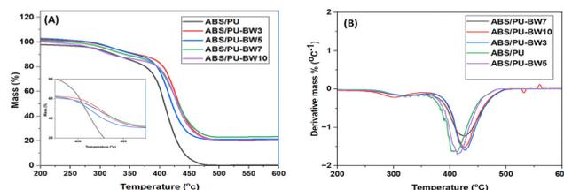
Fig. 6 (A) TGA curves of ABS/PU and ABS/PU–BW composite membranes, (B) DTG curves of ABS/PU and ABS/PU–BW composite membranes.
