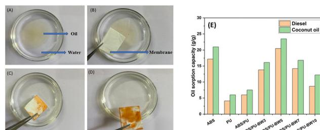
**Fig. 8** (A)–(D) Images of selective absorption of diesel from the water surface with ABS/PU–BW5 membranes. (E) Maximum oil absorption capacity of various concentrations of ABS/PU–BW membranes in diesel and coconut oil.
