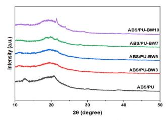
Fig. 4 X-Ray diffraction of the ABS/PU and ABS/PU-BW electrospun
