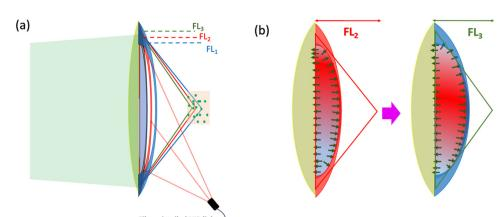
Fig. 1 Schematic of (a) the focusing property of the CsWO<sub>3</sub> NP solution-filled PDMS fluidic lens upon NIR irradiation and (b) the result of heat convection within the fluidic chamber that renders the transfer of heat through heat conduction from water medium to PDMS.
