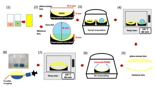
Fig. 2 Design and fabrication of the CsWO<sub>3</sub> NP solution-incorporated PDMS fluidic lens. A flow of the fabrication processes of the PDMS lens in a series of (1) PDMS preparation, (2) molding, (3) vacuuming, (4) thermal annealing, ((5), (6) and (7)) lens bonding, and (8) NP solution-filling processes is presented.
