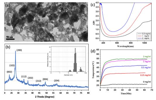
Fig. 4 Stoichiometric properties of CsWO<sub>3</sub> NPs. (a) TEM images of the NPs' contour profile and shape. (b) XRD spectrum the NP's crystallinity. (c) Optical absorbance and (d) temporally dependent increase in temperature as a function of the NP concentration. Optical power density used in (d) is 124 mW cm<sup>-2</sup>.
