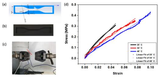
Fig. 5 Thermo-mechanical properties of PDMS. (a) Solidwork design, (b) 3D printed mold and (c) PDMS specimen attached to a strain gauge for the tensile test, and (d) the stress-strain plots with linearly fitting lines as a function of ambient temperature are presented.
