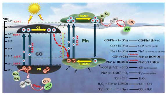
Fig. 13 Plausible photocatalytic mechanism of dye degradation by the GO/Pln composite: diagrammatic representation and proposed pathway scheme
