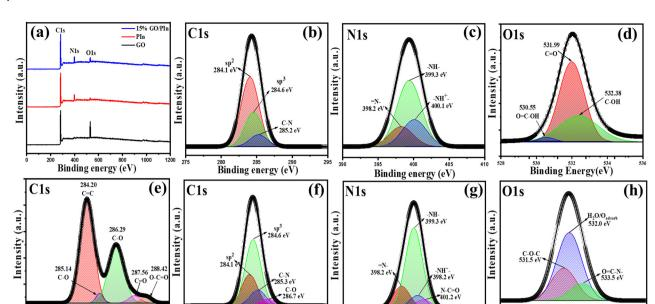
Fig. 6 XPS (a) survey spectra of GO, Pln and 15%GO/Pln. High-resolution spectra: (b) C 1s and (c) N 1s of Pln; (d) O 1s and (e) C 1s of GO; (f) C 1s, (g) N 1s and (h) O 1s of 15%GO/PIn
