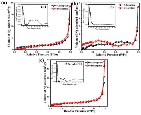
Fig. 7 N<sub>2</sub> adsorption-desorption isotherms of (a) GO, (b) Pln, and (c) 15%GO/Pln (insets: Barrett-Joyner-Halenda (BJH) pore size vs. pore volume distribution plots for the respective N2 sorption isotherms).
