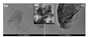
Fig. 5 TEM images of (a) GO, (b) PIn and (c) 15%GO/PIn composite.
