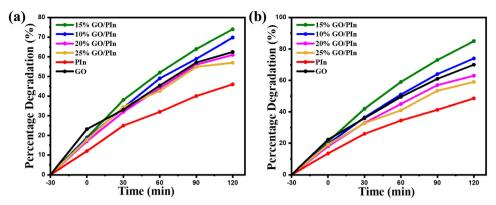
Fig. 9 Photocatalytic degradation graphs of (a) AO and (b) EY dye using GO, Pln and GO/Pln nanocomposites.
