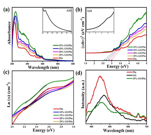
Fig. 3 (a) UV-visible spectra, (b) Tauc plots for Pln and composites (insets: GO absorbance spectra and Tauc plot, respectively), (c) Urbach energy plots for Pln and composites, and (d) PL spectra of GO, Pln and 15%GO/Pln composite.
