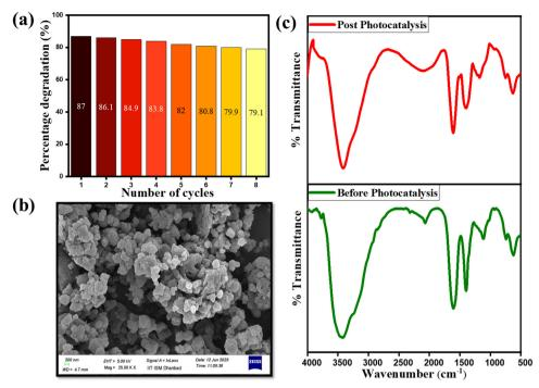
Fig. 14 (a) Recyclability studies of the 15%GO/Pln composite for FB dye degradation. Post-photocatalytic (b) FESEM image and (c) FTIR spectra of the 15%GO/Pln composite before and after eight cycles.
