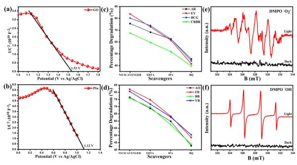
Fig. 12 Mott-Schottky plots of (a) GO and (b) PIn. Scavenger studies of (c) anionic and (d) cationic dyes. ESR spectra of (e) DMPO- ${}^{\bullet}$ O<sub>2</sub> and (f) DMPO- ${}^{\bullet}$ OH.
