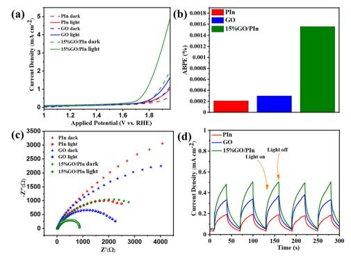
Fig. 8 (a) Polarisation curves obtained from linear sweep voltammetry measurements. (b) Bar diagram representing an applied bias photon-to-current efficiency of 1.2 V vs. RHE. (c) Nyquist plot obtained from electrochemical impedance spectroscopy measurements. (d) Transient photocurrent response in the dark and under illumination at 1.6 V vs. RHE
