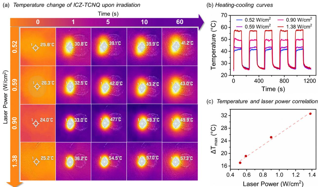
Fig. 4 (a) Thermal IR images of **ICZ-TCNQ** under heating at different times and density power. (b) Heating-cooling curves for **ICZ-TCNQ**. (c) Linear relationship between change in temperature and the applied laser power.
