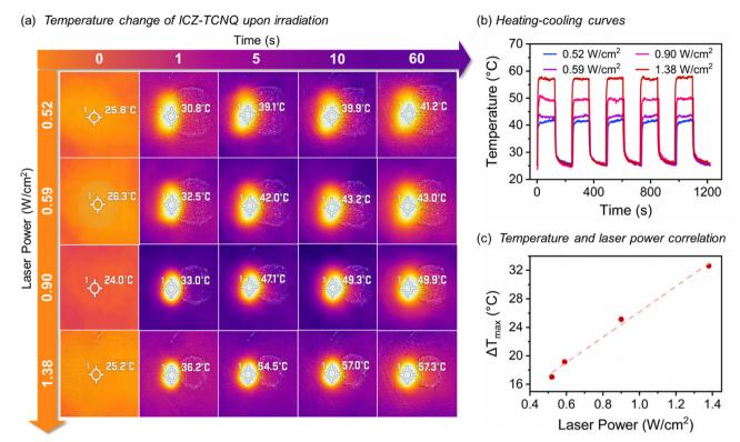
Fig. 4 (a) Thermal IR images of ICZ-TCNQ under heating at different times and density power. (b) Heating-cooling curves for ICZ-TCNQ. (c) Linear relationship between change in temperature and the applied laser power.
