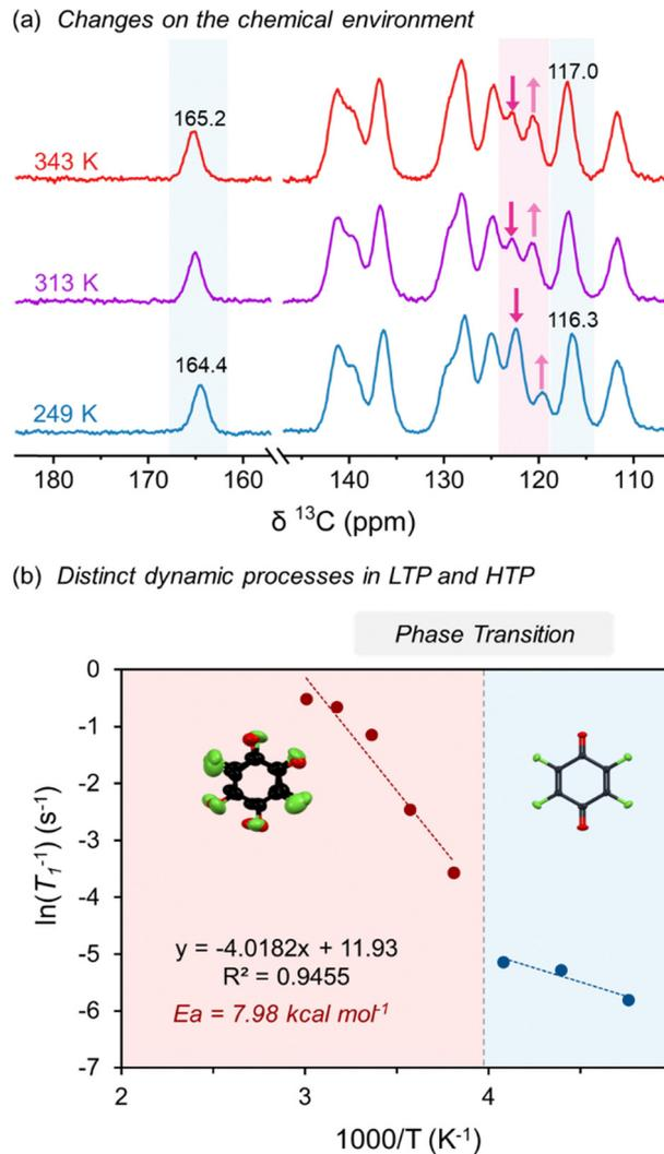
Fig. 7 (a) <sup>13</sup>C CPMAS spectra of ICZ-TFBQ at three different temperatures. (b) Arrhenius fitting of the <sup>19</sup>F  $T_1$  relaxation times obtained from saturation recovery experiments.
