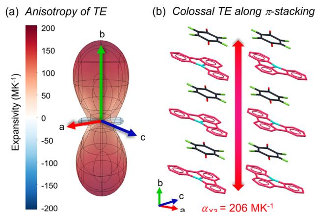
Fig. 6 (a) Expansivity indicatrix for **ICZ-TFBQ**. (b) Crystalline packing of **ICZ-TFBQ** seen along the  $b$ -axis in the direction of the  $\pi$ -stacking between D/A molecules. The TE coefficient is displayed and illustrated with red arrows.
