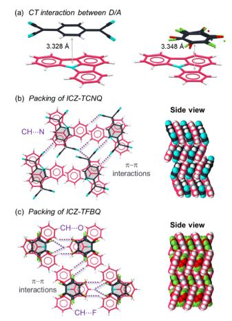
Fig. 2 (a) Interplanar distances between donor and acceptor molecules in **ICZ-TCNQ** (left) and **ICZ-TFBQ** (right). Intermolecular  $\pi - \pi$  (grey) and hydrogen bond (purple) interactions in (b) ICZ-TCNQ cocrystal and (c) ICZ-TFBQ cocrystal with their respective packing.
