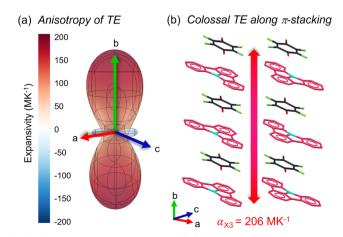
Fig. 6 (a) Expansivity indicatrix for ICZ-TFBQ. (b) Crystalline packing of **ICZ-TFBQ** seen along the *b*-axis in the direction of the  $\pi$ -stacking between D/A molecules. The TE coefficient is displayed and illustrated with red arrows.
