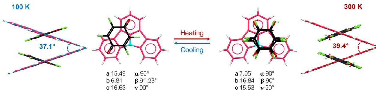
Fig. 5 Molecular structure differences between the LTP and HTP polymorphs in **ICZ-TFBQ**. (a) Phase transition from ordered to disordered **TFBQ** molecules depending on temperature. (b) Changes of the packing angles of the aromatic donor cores of **ICZ-TFBQ** from LTP to HTP and displacement of the atomic positions of the **TFBQ**.
