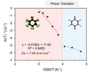
Fig. 7 (a)  $^{13}$ C CPMAS spectra of **ICZ-TFBQ** at three different temperatures. (b) Arrhenius fitting of the  $^{19}$ F  $T_1$  relaxation times obtained from saturation recovery experiments.
