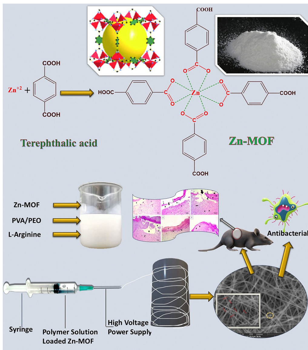
Fig. 1 Schematic illustration of the preparation of Zn-MOF and PVA/PEO/L-Arg/Zn-MOF NFs and their possible antibacterial and tissue regeneration capacity, further leading to promoting wound healing.
