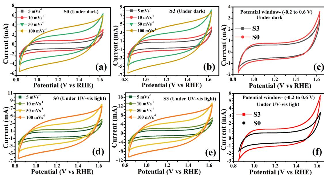
Fig. 6 Scan rate CV curves of S0 and S3 electrodes (active material  $\sim 1\text{ mg}$ , area  $\sim 0.5\text{ cm}^2$ ) under dark (a–c) and UV-vis light (d–f) irradiation (250 W Hg-lamp) in a 0.5 M aqueous  $\text{Na}_2\text{SO}_4$  electrolyte. Applied scan rate is  $5\text{ mV s}^{-1}$  (Fig. 6c and f).
