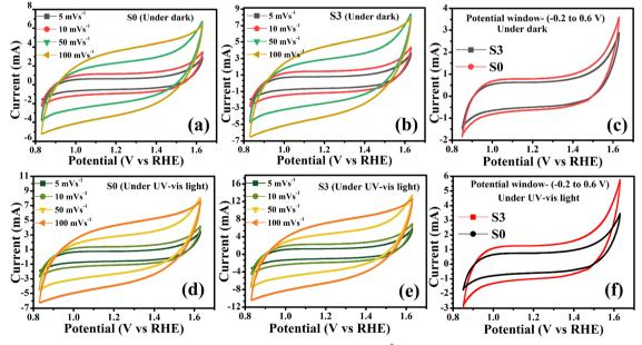
Fig. 6 Scan rate CV curves of S0 and S3 electrodes (active material  $\sim$ 1 mg, area  $\sim$ 0.5 cm<sup>2</sup>) under dark (a–c) and UV-vis light (d–f) irradiation (250 W Hg-lamp) in a 0.5 M aqueous Na<sub>2</sub>SO<sub>4</sub> electrolyte. Applied scan rate is 5 mV s<sup>-1</sup> (Fig. 6c and f).
