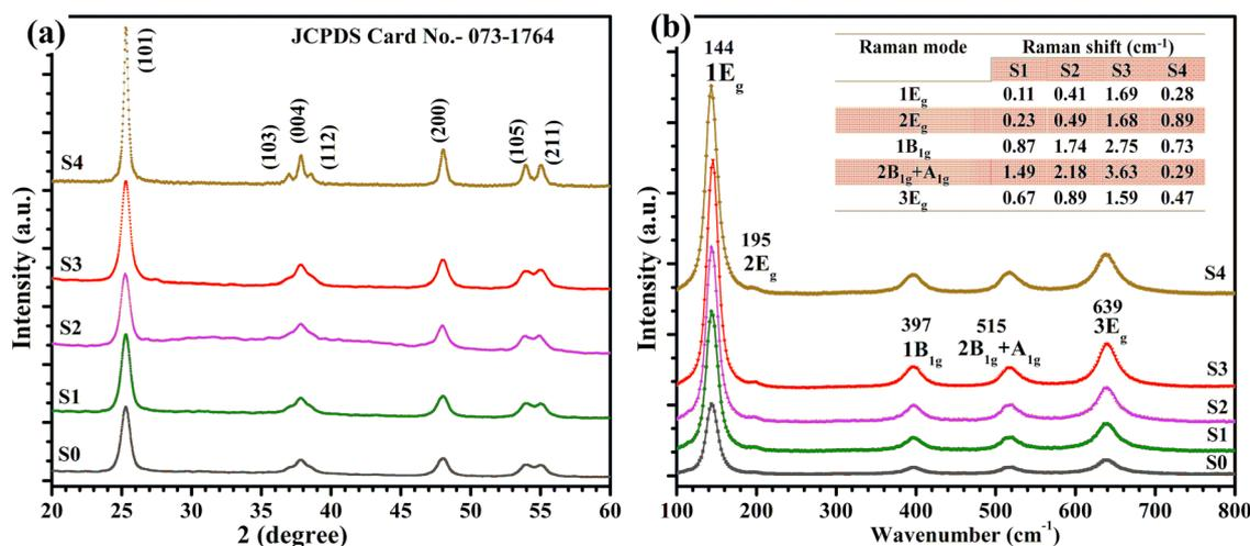
Fig. 1 Indexed XRD pattern (a) and Raman spectra (b) of as-synthesized powder samples. Pristine anatase TiO<sub>2</sub> (S0) and Cu-doped TiO<sub>2</sub> (1%-S1, 2%-S2, 3%-S3, 4%-S4). Insets in (b) are Raman shifts in S3 with respect to S0.
