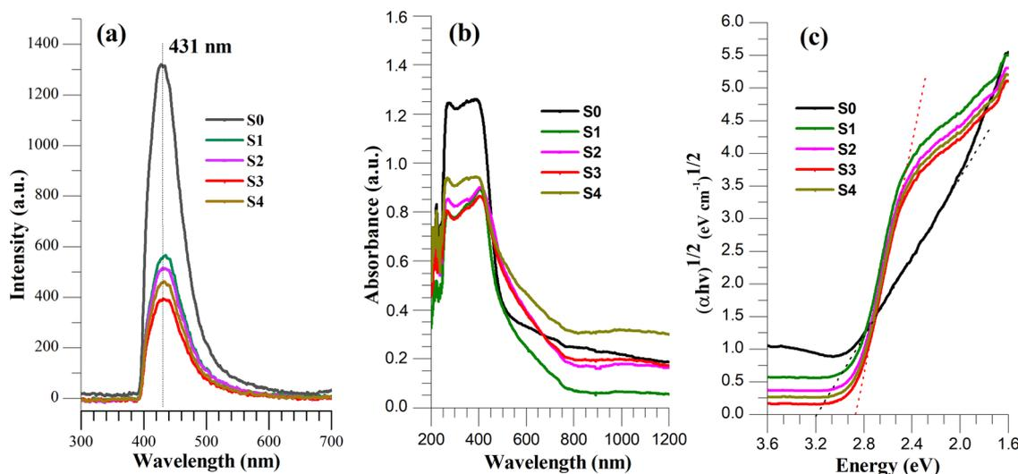
**Fig. 2** PL spectra (a) of all powders, highlighting that the S3 sample has the least recombination of charge pairs. Optical absorption spectra (b) and Tauc  $[(\alpha hv)^{1/2}$  vs.  $hv$ ] plots (c) for samples.
