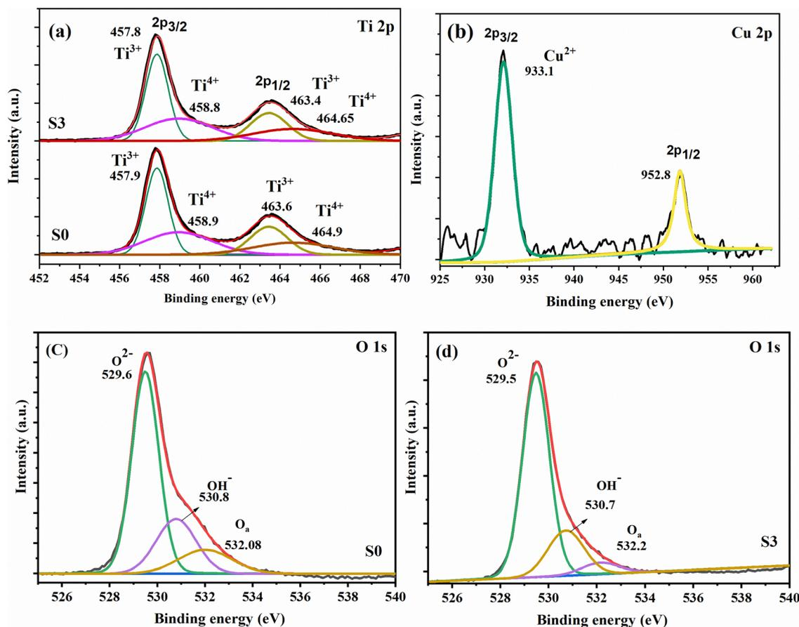
Fig. 4 High-resolution XPS spectra of (a) Ti, (b) Cu, and (c–d) O (lattice oxygen  $\rightarrow$  O<sup>2-</sup>; surface hydroxy radicals  $\rightarrow$  OH<sup>-</sup>; surface adsorbed oxygen  $\rightarrow$  O<sub>s</sub>) of S0 and S3 samples. A BE of  $\sim$ 284.6 eV for the surface adventitious C1s peak is used as a calibrating reference.
