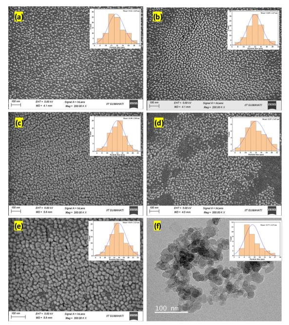
Fig. 4 FESEM micrographs of FMZ samples: (a) FZ, (b) FMZ0.25, (c) FMZ0.5, (d) FMZ0.75, and (e) FM. (f) FETEM micrograph and particle distribution of the FMZ0.75 sample.
