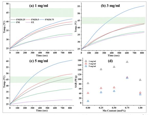
Fig. 6 Increase in the temperature of the medium through the heat generated by FMZ nanoparticles at concentrations of (a) 1 mg mL $^{-1}$ , (b) 3 mg mL $^{-1}$ . and (c) 5 mg mL<sup>-1</sup> when subjected to an alternating magnetic field, and (d) influence of Mn content on the specific absorption rate values estimated for the FMZ samples
