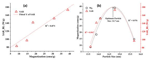
Correlation between (a) magnetization and SAR values and (b) particle size and magnetization and SAR values.
