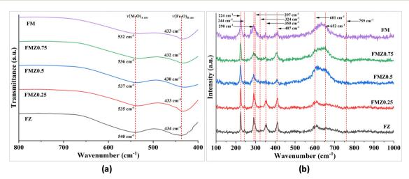
Fig. 2 (a) FTIR and (b) Raman spectra of Mn- and Zn-doped ferrite nanoparticles illustrating their chemical functional groups.
