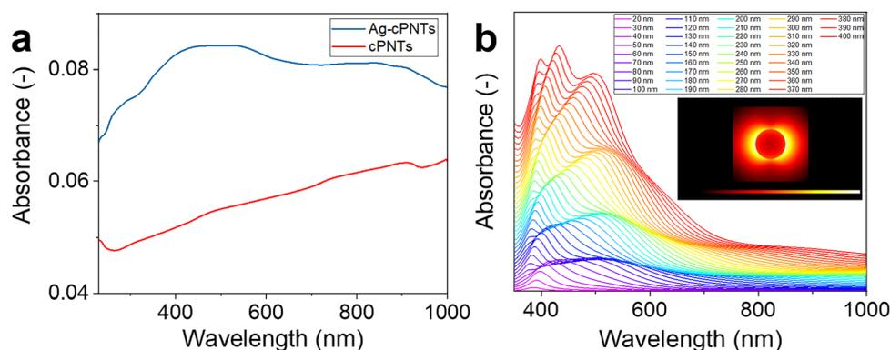
Fig. 2 (a) Measured UV-Vis spectra of the carbonized polypyrrole nanotubes with (blue curve) and without AgNPs (red one); (b) calculated UV-Vis spectra of pristine AgNPs depending on their size; the inset shows the simulated photoexcited local plasmon-related electric field.
