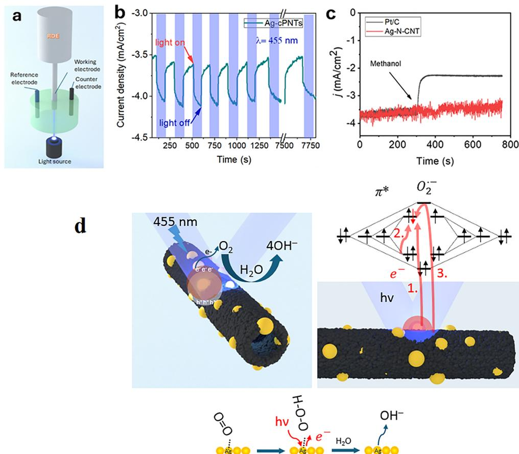
Fig. 4 (a) Schema of the custom-made electrochemical setup for plasmon-enhanced material properties; (b) chronoamperometric  $I-t$  measurements of the Ag nanoparticle-decorated N-doped carbonized polypyrrole nanotubes (Ag-cPNTs) with 455 nm LED light on and off; (c) methanol tolerance test; (d) possible mechanisms of AgNP-decorated N-doped carbon nanotubes.
