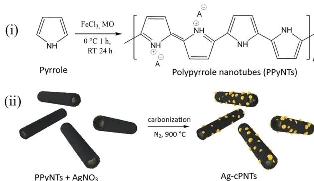
**Scheme 1** Illustration of plasmon-active Ag-cPNT composite preparation: (i) synthesis of polypyrrole nanotubes (PPyNTs) and (ii) addition of AgNO<sub>3</sub> with subsequent carbonization under nitrogen flow.
