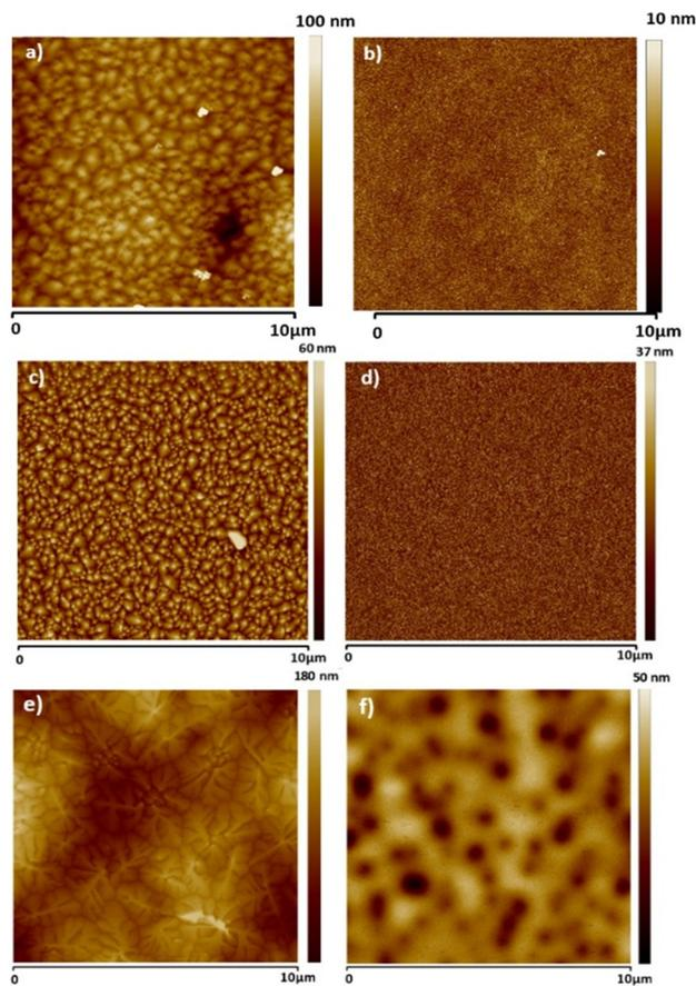
Fig. 12 AFM scans of the semiconductors grown on the dielectric capping layer. (a) Pentacene on larch, (b)  $C_{60}$  on larch; (c) pentacene on Atlas cedar, (d)  $C_{60}$  on Atlas cedar; (e) pentacene on spruce and (f)  $C_{60}$  on spruce.
