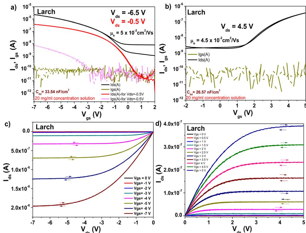
Fig. 13 Transistor measurements of Larch resin on  $\sim 17$  nm thick  $\text{Al}_2\text{O}_3$  gate with pentacene and  $\text{C}_{60}$  as organic semiconductors. (a) Transfer curve of the OFET using pentacene as the organic semiconductor. (b) Transfer curve of the OFET using  $\text{C}_{60}$  as the organic semiconductor. (c) Output curve of the OFET using pentacene as the organic semiconductor. (d) Output curve using  $\text{C}_{60}$  as the organic semiconductor.
