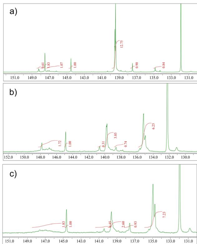
**Fig. 3**  $^{31}\text{P}$  NMR spectra in the 130–150 ppm region recorded for (a) larch, (b) Atlas cedar, and (c) spruce after derivatization of the resins with TMDP. The 132.2 ppm signal was derived from the reaction of residual TMDP with water and used for the calibration of the chemical shifts.
