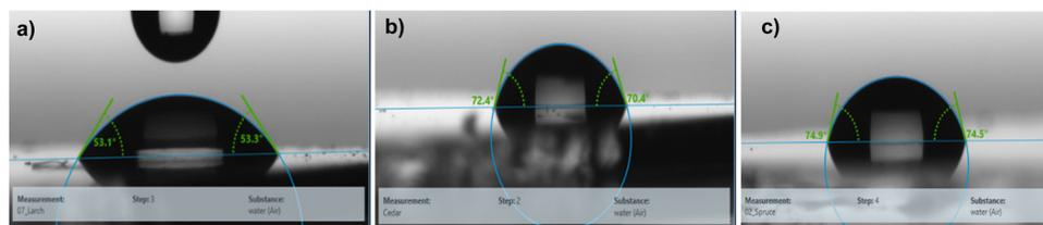
Fig. 6 Water droplet contact angle of (a) larch resin; (b) Atlas cedar resin; and (c) spruce resin.
