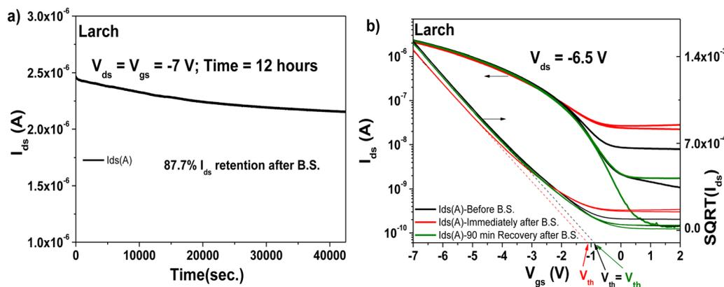
Fig. 14 OFET with Larch resin and pentacene semiconductor evaluated for bias stress stability: (a) bias stress measurement curve after applying constant voltages to the OFET device,  $V_{ds} = V_{gs} = -7$  V for 12 hours. (b) Recovery of the transistor characteristics after the bias stress measurements.
