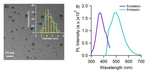
Fig. 1 (A) High-resolution transmission electron microscopy (HRTEM) image of Trp-Cu NCs. The inset shows the corresponding size distribution (number of particles analysed (N) = 110) obtained from the HRTEM image. (B) Excitation ( $\lambda_{em}$  = 500 nm) (violet) and emission ( $\lambda_{ex}$  = 380 nm) (cyan) spectra of Trp-Cu NC.
