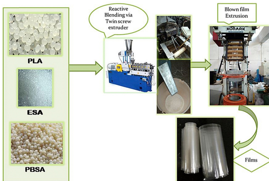
Fig. 14 Schematic of the processing steps for PLA/PBSA/ESA blend-based films: dry blending and blown film extrusion. Reproduced from ref. 219 with permission from Elsevier, copyright 2020.
