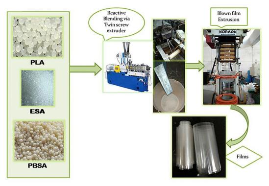
Fig. 14 Schematic of the processing steps for PLA/PBSA/ESA blend-based films: dry blending and blown film extrusion. Reproduced from ref. 219 with permission from Elsevier, copyright 2020
