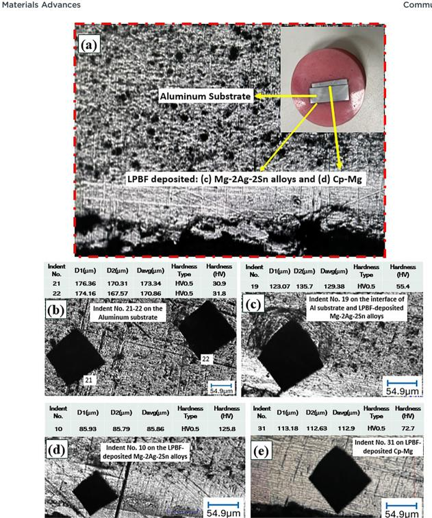
Fig. 4 (a) Cross-sectional view of LPBF printed circular Mg-2Ag-2Sn and Cp-Mg samples on an aluminium substrate; hardness measurement on the (b) aluminum substrate and (c) interface of the substrate and the LPBF printed Mg-2Ag-2Sn alloy, (d) the LPBF printed Mg-2Ag-2Sn alloy, and (e) LPBF printed Cp-Mg.
