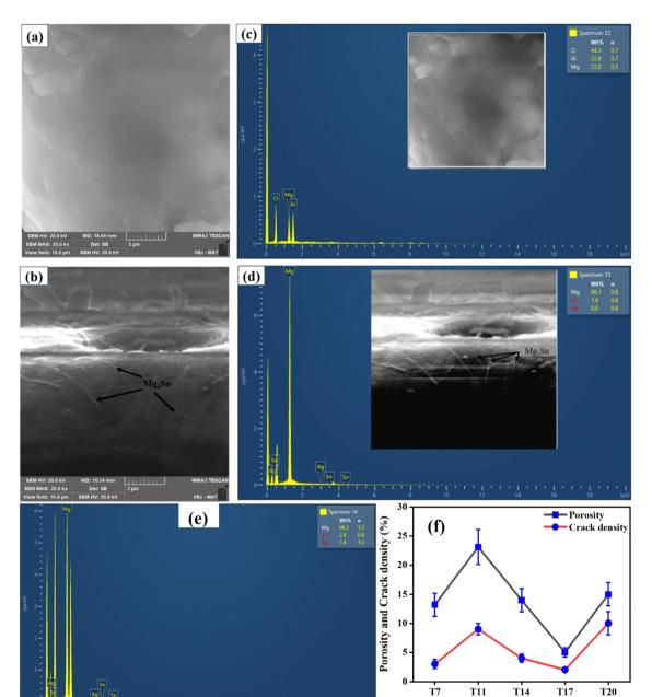
Fig. 3 (a) and (b) SEM micrographs of Cp-Mg and Mg-2Ag-2Sn alloys, respectively, and (c)-(e) their corresponding EDS spectra of alloy (f) porosity and crack density vs. track number plot for different tracks.
