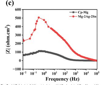
Fig. 5 (a) Tafel plot, (b) Nyquist plot, and (c) Bode plot of Cp-Mg and Mg-2Ag-2Sn circular samples prepared at optimized process parameters (T17).
