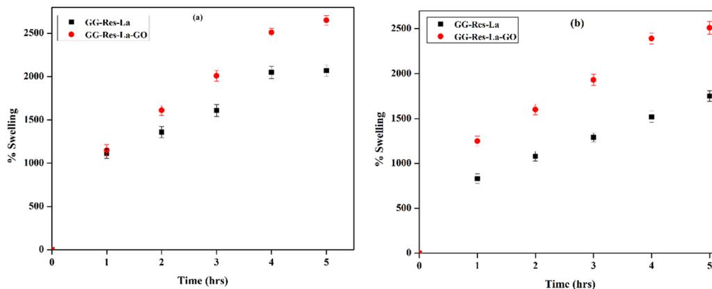
Fig. 9 Swelling in (a) NaCl and (b) CaCl<sub>2</sub> solutions.
