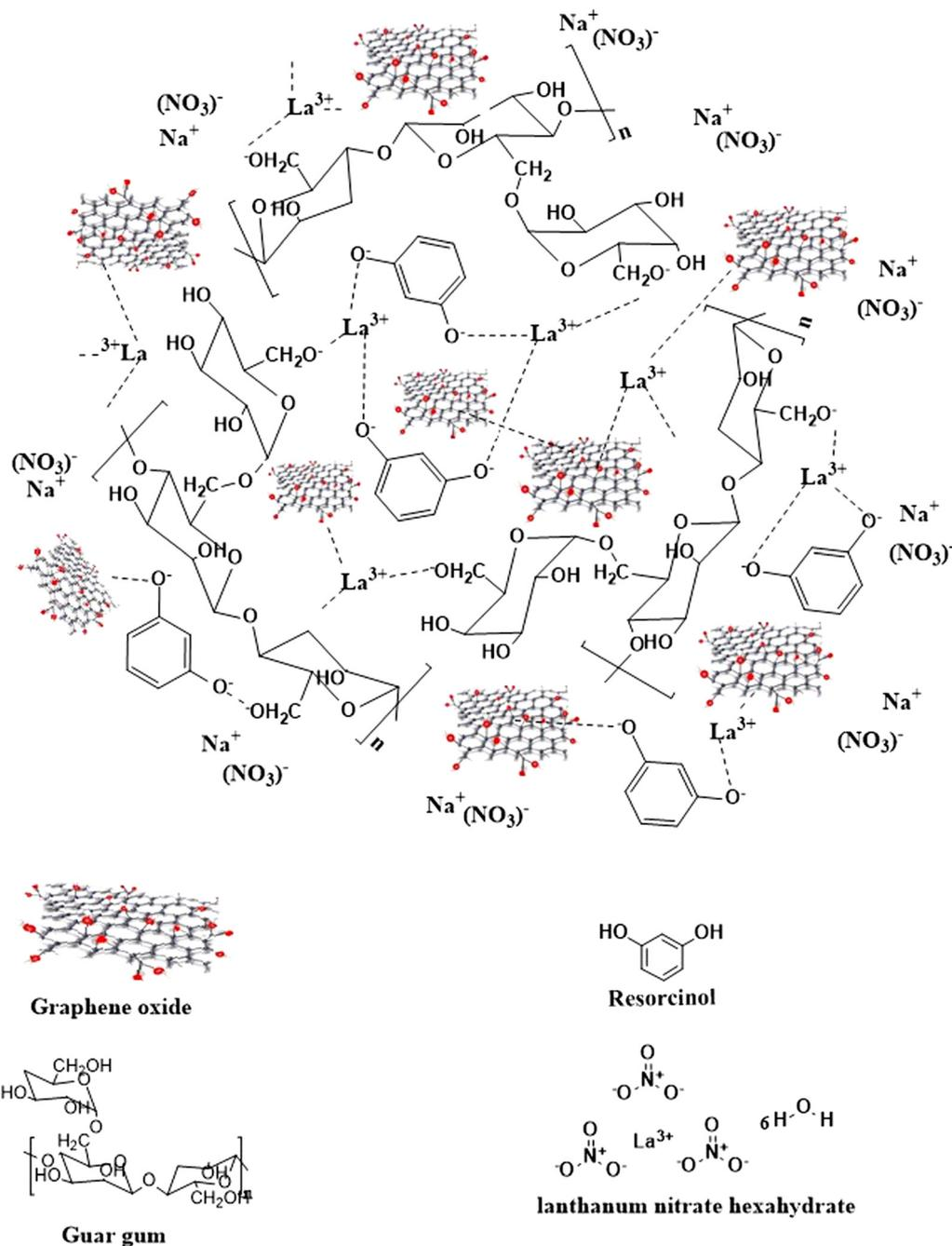
Scheme 1 Possible mechanistic interactions in the prepared hydrogel beads under alkaline conditions.
