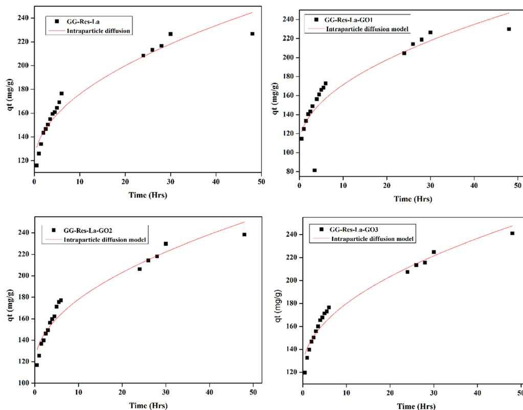
Fig. 19 Intra-particle diffusion kinetics of hydrogels at pH 9.
