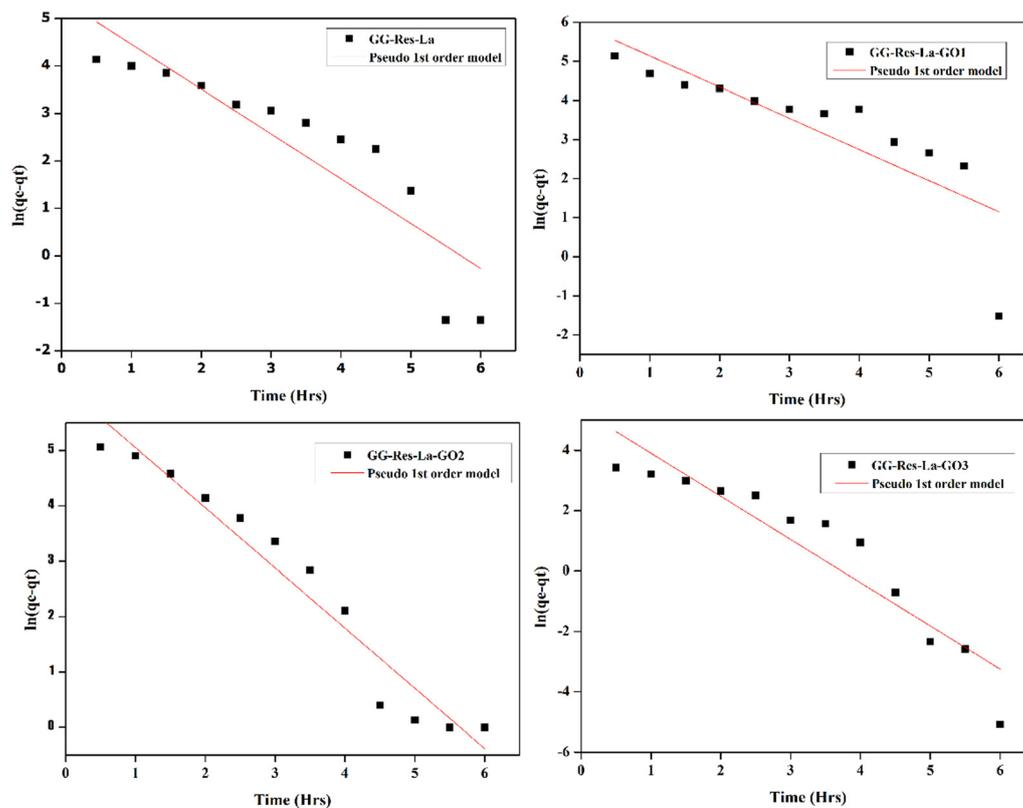
Fig. 14 Pseudo-first-order kinetic model of hydrogels in water.
