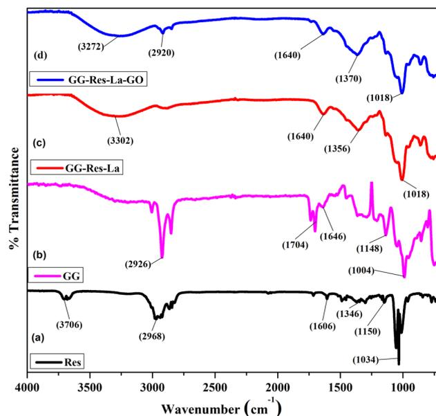
Fig. 4 FTIR spectra of the prepared hydrogel beads.
