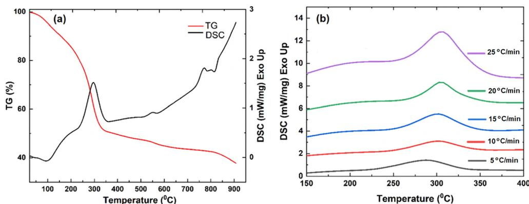
Fig. 1 TG-DSC curves of the  $\text{Yb}^{3+}/\text{Er}^{3+}$ -doped  $\text{SiO}_2$ - $\text{GdF}_3$  xerogel co-doped with Li, measured in synthetic air at a heating rate of  $10^\circ\text{C min}^{-1}$  (a) and the crystallization peak highlighted at five different heating rates: 5, 10, 15, 20, and  $25^\circ\text{C min}^{-1}$  (b).
