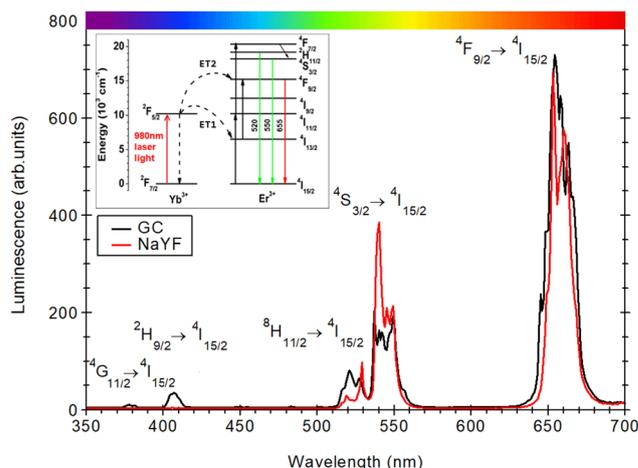
Fig. 5 Normalized UC luminescence spectra recorded for GCLiYb/Er glass-ceramic (after calcination at 525 °C) and  $\beta\text{-NaYF}_4\text{:18Yb/2Er}$  polycrystalline powder recorded under 980 laser light pumping and the possible mechanism with the RE energy levels involved (inset).
