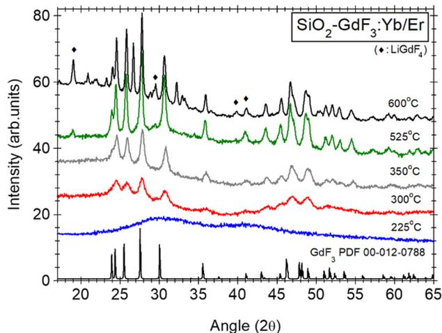
Fig. 2 XRD patterns of GCLiYb/Er glass-ceramic samples after annealing at different temperatures; the XRD pattern of orthorhombic  $\text{GdF}_3$  (PDF 012-0788) is included.
