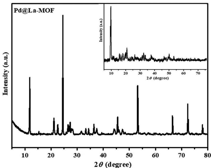
Fig. 2 X-ray diffraction (XRD) pattern of the Pd@La-BDC MOF nanocomposite (inset: La-BDC MOF); the XRD pattern confirms the crystalline structure and successful incorporation of Pd into the La-BDC MOF, with well-defined peaks indicating maintained structural integrity and phase purity.
