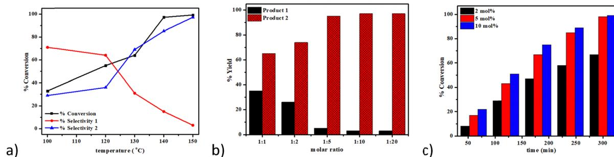
Fig. 8 Optimization of the reaction conditions for the Pd@La-BDC MOF-catalyzed *N*-benzylation reaction: (a) effect of temperature variation; (b) influence of varying molar ratios of reactants (aniline : benzyl alcohol); and (c) impact of different catalytic dosages.
