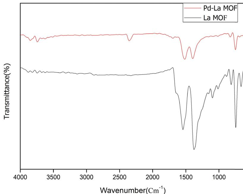
Fig. 1 FTIR spectra of the synthesized Pd@La-BDC and La-BDC MOFs; the spectra reveal shifts in the carboxylate and M–O bond vibrations upon Pd incorporation into La-BDC, confirming successful synthesis and structural modification of the Pd@La-BDC MOF.
