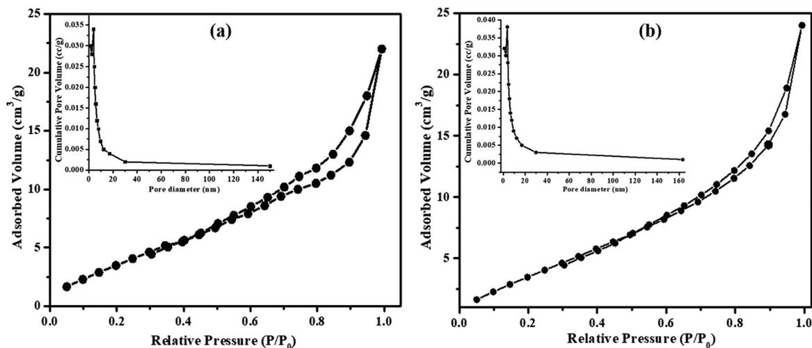
Fig. 5  $N_2$  adsorption–desorption isotherms of the (a) La-BDC MOF and (b) Pd@La-BDC MOF nanocomposite, with the inset showing pore size distribution, demonstrating the material's high surface area and porosity.
