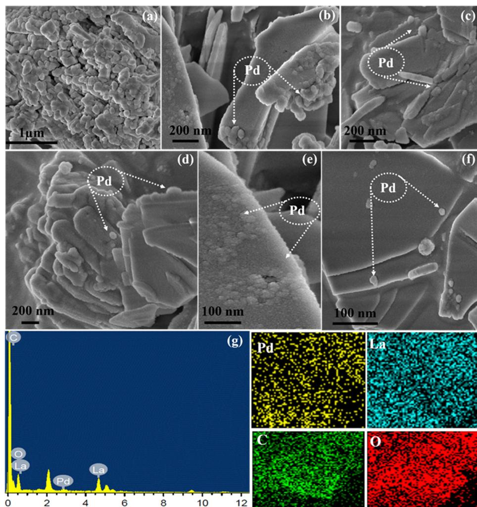
**Fig. 3** (a) The FESEM image of the pristine La-BDC MOF shows a uniform morphology; (b)–(f) FESEM images of the Pd@La-BDC MOF nanocomposite illustrate successful Pd incorporation, with morphological changes; (g) EDS analysis confirms the presence and uniform distribution of Pd and other constituent elements in the nanocomposite.
