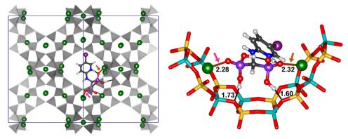
Fig. 4 Left: DFT-optimized lowest-energy configuration of BP6 in CaX. For clarity, the zeolite framework is displayed using grey tetrahedra, Ca<sup>2+</sup> cations are shown as green spheres. Ca. O bonds are highlighted with arrows, hydrogen bonds are shown as light black lines. Projection along [110]. Right: Zoomed-in view of the local environment of BP6, emphasizing close contacts to framework atoms. The Ca...O and hydrogen bond distances are given in Å.
