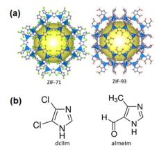
Fig. 1 (a) RHO topology of ZIF-93 and ZIF-71. ZnN<sub>4</sub> tetrahedra are shown in blue, and the yellow spheres indicate empty spaces in the cage. Linkers are shown in ball and stick representation (H in pink, C in grey, N in blue, O in red and Cl in green). (b) The structure of 4,5-dichloroimidazole (dcllm) and 4-methyl-5-imidazolecarboxaldehyde (almelm), which are the linkers for ZIF-71 and ZIF-93, respectively
