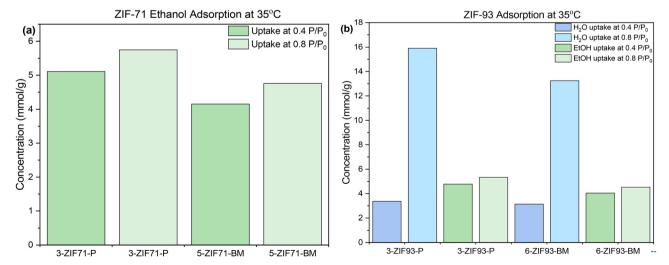
Fig. 9 Bar charts showing (a) ethanol uptake of ZIF-71, and (b) ethanol and water uptake of ZIF-93 obtained at 35 °C, with data for 0.4 P/P<sub>0</sub> and 0.8 P/P<sub>0</sub>.
