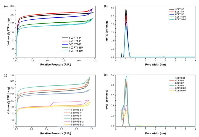
Nitrogen physisorption isotherms and pore size distributions of the activated (a, b) ZIF-71 and (c, d) ZIF-93 samples.
