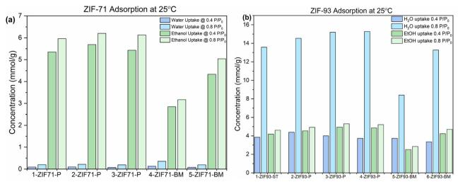
Fig. 8 Bar charts showing the ethanol and water uptake for (a) ZIF-71 and (b) ZIF-93 obtained at 25 °C, showing data for 0.4 P/P<sub>0</sub> and 0.8 P/P<sub>0</sub>
