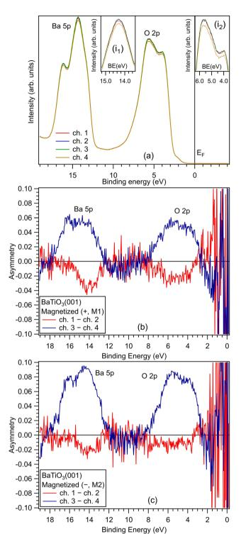
Fig. 4 Valence band spin-resolved photoelectron spectroscopy, obtained with a photon energy of 105 eV. (a) Signals obtained for the different spin-resolved channels (Fig. 3(b)). Insets (i $_1$ ) and (i $_2$ ) are magnified areas of the maxima corresponding to Ba 5p and O 2p states, respectively. (b) and (c) show the spin asymmetry detected for the sample subject to the M1 or M2 magnetization process, as represented in Fig. 3(a).
