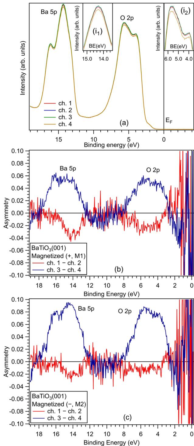
Fig. 4 Valence band spin-resolved photoelectron spectroscopy, obtained with a photon energy of 105 eV. (a) Signals obtained for the different spin-resolved channels (Fig. 3(b)). Insets ( $i_1$ ) and ( $i_2$ ) are magnified areas of the maxima corresponding to Ba 5p and O 2p states, respectively. (b) and (c) show the spin asymmetry detected for the sample subject to the M1 or M2 magnetization process, as represented in Fig. 3(a).
