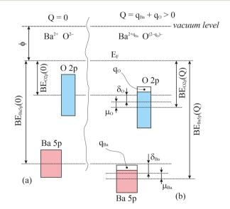
(a) Position of completely filled O 2p and Ba 5p bands in a bulk  ${\sf Ba}^{2+}{\sf O}^{2-}$  layer. (b) Position of partially filled O 2p and Ba 5p bands in a surface charged  $Ba^{(2+qBa)}^{\dagger}O^{(2-qO)}$  layer, with  $q_{Ba}+q_{O}=Q$ , the total charge per surface unit cell.  $\delta_{\mathsf{Ba},\mathsf{O}}$  are chemical shifts due to additional charges on each type of ion, and  $\mu_{Ba,O}$  are shifts due to the surrounding crystal fields.
