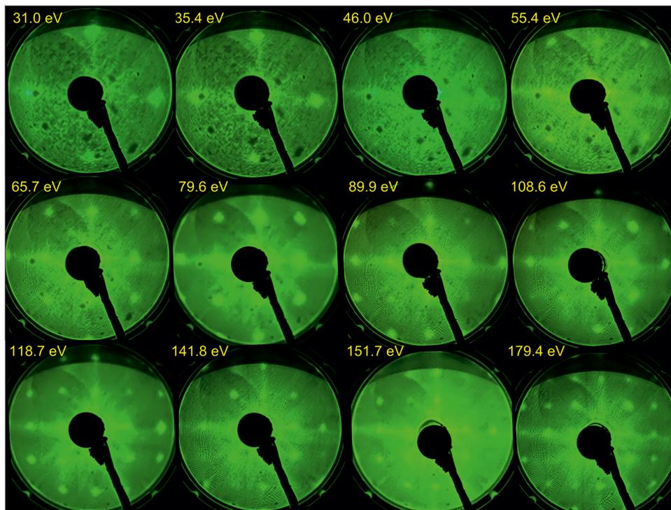
Fig. 1 Low-energy electron diffraction (LEED) images of BaTiO<sub>3</sub>(001), after preparation under ultra-high vacuum conditions. Each image indicates the kinetic energy of the electrons.
