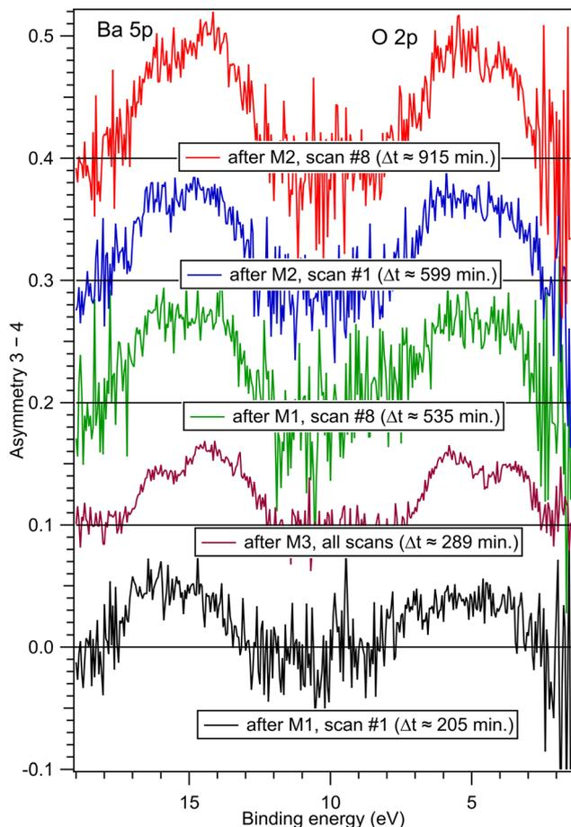
Fig. 6 Time evolution of the recorded spin asymmetry between spin channels 3 and 4 during individual scans (46 min each) together with the corresponding signal of the M3 experiment. For each signal, an estimate of the time elapsed from the end of the sample preparation is given.
