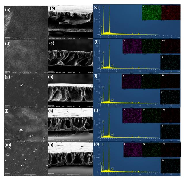
Fig. 2 SEM images of the surface and cross-section, along with EDX and elemental mapping of membranes: (a-c) M1, (d-f) M2, (g-i) M3, (j-l) M4, and (m-o) M5.
