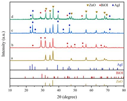
Fig. 3 XRD patterns of ZnO/BiOI/Agl. (a) ZnO, (b) ZnO/BiOI, (c) ZnO/Agl and (d) ZnO/BiOI/Agl.
