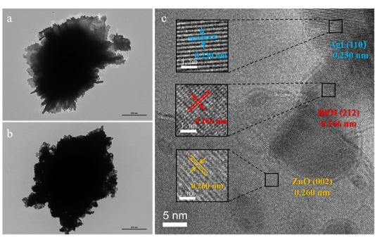
Fig. 2 The TEM images of (a) ZnO and (b) ZnO/BiOI/AgI. (c) HRTEM image of ZnO/BiOI/AgI.
