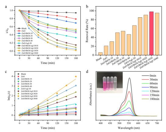
Fig. 9 Photocatalytic activity of different materials for NOR antibiotics under visible light. (a) Degradation curve of NOR antibiotics. (b) Degradation rate of NOR with different ratios of materials. (c) First-order kinetics for the photocatalytic degradation of NOR. (d) Time-resolved UV-vis absorbance spectra for the photocatalytic degradation of NOR antibiotics by the ZnO/BiOI/AgI-3030 sample at 30-minute intervals.
