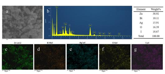
(a) and (b) EDS spectrum of ZnO/BiOI/AgI. (c)–(g) EDS elemental mapping of Zn, Bi, Ag, O and I in ZnO/BiOI/AgI.
