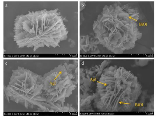
Fig. 1 The SEM images of (a) ZnO, (b) ZnO/BiOI, (c) ZnO/AgI and (d) ZnO/BiOI/AgI.
