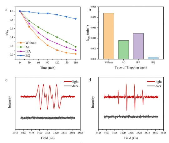
Fig. 13 The effect of reactive oxygen species on photocatalysis. (a) Degradation curves of RhB with different free radical trapping agents. (b) Degradation rate of RhB in free radical trapping experiments. (c) ESR spectrum of  ${}^{\bullet}O_2^{-}$  labeled by DMPO. (d) ESR spectrum of  ${}^{\bullet}OH$  labeled by DMPO.
