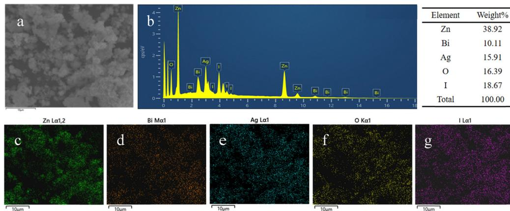
Fig. 5 (a) and (b) EDS spectrum of ZnO/BiOI/AgI. (c)–(g) EDS elemental mapping of Zn, Bi, Ag, O and I in ZnO/BiOI/AgI.
