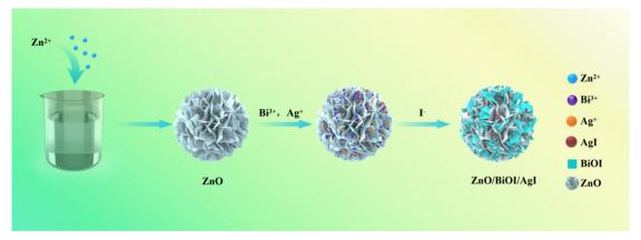
Scheme 1 Preparation process of ZnO/BiOI/AgI nanocomposites.
