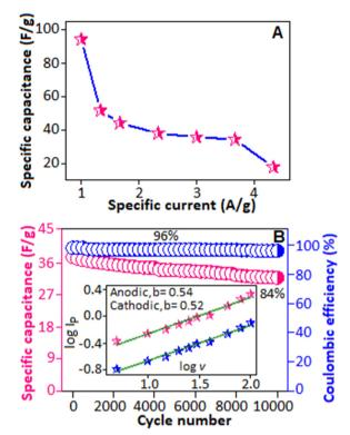
Fig. 10 (A) Graphical representation of specific capacitance as a function of specific current. (B) Specific capacitance and coulombic efficiency of the device at 3.0 A  $\rm g^{-1}$  for 10 000 GCD cycles (upper panel). Linear fitting of the anodic and cathodic peak currents (lower panel).
