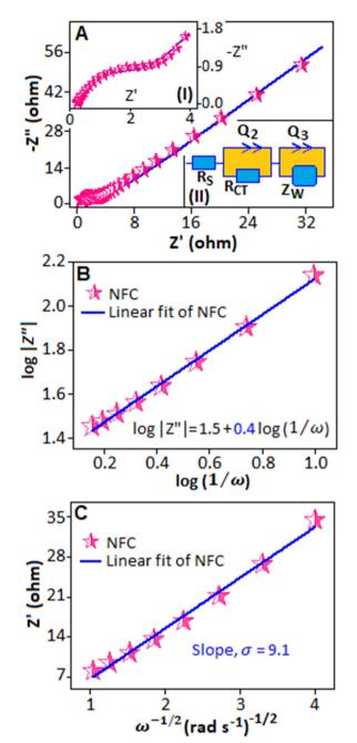
Fig. 8 (A) Nyquist plot of the NFC-modified electrode. Inset (I): magnified image of the Nyquist plot for the high-frequency region; inset (II): the equivalent circuit model. (B) Graphical representation of  $\log |Z''| \ vs. \log(1/\omega)$ . (C) Graphical representation of Z' (Ohm)  $vs. \ \omega^{-1/2}$  (rad  $s^{-1})^{-1/2}$ .
