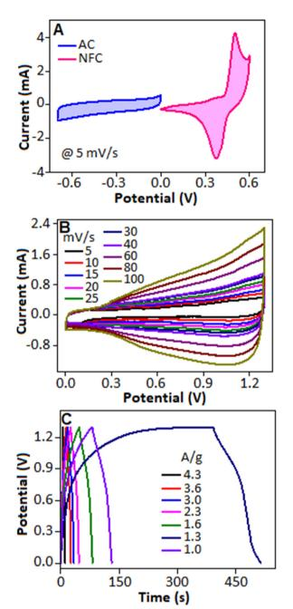
Fig. 9 (A) Comparative CV profiles of AC- and NFC-modified electrodes at 5 mV s<sup>-1</sup>. (B) Voltammograms of the hybrid device under various scan rates in the range of 5–100 mV s<sup>-1</sup>. (C) Galvanostatic charge-discharge profile of the device under various current densities ranging from 4.3 to  $1.0 \text{ A g}^{-1}$
