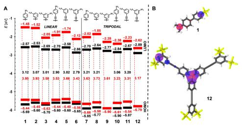
Fig. 3 Energy level diagram of chromophores **1–12** showing electrochemical (black) and DFT-calculated (red) energies of the frontier molecular orbitals (A) and the HOMO (red) and the LUMO (blue) localizations in representative chromophores **1** and **12** (B).
