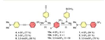
Scheme 1 Synthesis of linear  $SF_5$ -capped chromophores 1-6. (i)  $[PdCl_2(PPh_3)_2]$ ,  $Na_2CO_3$ ,  $THF/H_2O$  (4:1), 60 °C, 16 h; (ii)  $[PdCl_2(PPh_3)_2]$ , Cul, THF/TEA (4:1), 60 °C, 16 h.
