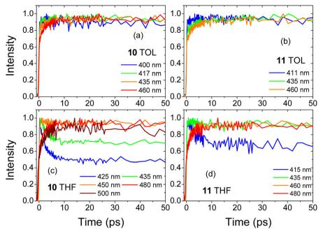
Fig. 7 Fluorescence up conversion dynamics in the ps timescale in TOL for (a) 10 and (b) 11 and in THF for 10 (c) and 11 (d) exc.: 380 nm, det.: at various emission wavelengths as shown in the figure.
