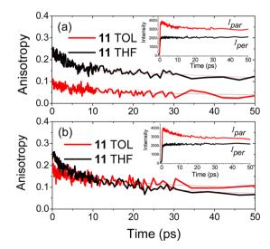
Fig. 8 Time resolved anisotropy dynamics in the ps timescale for 10 and 11 in TOL and THF, exc.: 380 nm, det.: at the peak of the emission spectra. The insets show the fluorescence dynamics detected at a parallel and perpendicular polarization for 10 (a) and 11 (b) in THF respectively.
