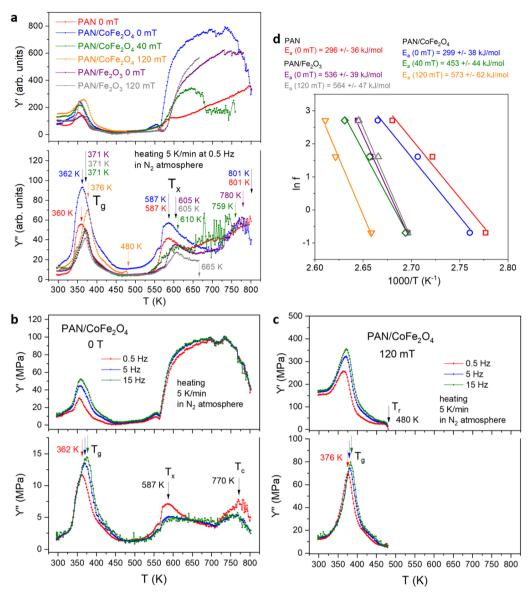
Fig. 5 (a) Dynamic mechanical analysis comparison of the investigated PAN, PAN/Fe<sub>2</sub>O<sub>3</sub> and PAN/CoFe<sub>2</sub>O<sub>4</sub> (for 0 T, 40 mT and 120 mT) at 5 K min<sup>-1</sup> heating rate between 300 K and 800 K. Frequency dependence of PAN/CoFe<sub>2</sub>O<sub>4</sub> at (b) 0 T and (c) 120 mT. (d) Activation energies for the PAN, PAN/Fe<sub>2</sub>O<sub>3</sub> and PAN/CoFe<sub>2</sub>O<sub>4</sub> samples at various magnetic fields.
