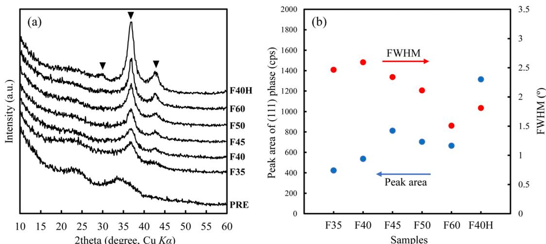
Fig. 1 (a) XRD patterns of the precursor film (**PRE**), UV-irradiated film (**FX**, X = controlled humidity in the range of 35–60%), and **F40H** obtained by heat treatment of **F40**. Triangles (▼) denote the crystal phases of  $\text{Cu}_2\text{O}$  (ICDD card no. 01-078-5772). (b) Peak area and FWHM of the  $\text{Cu}_2\text{O}$ (111) phase in **FX** and **F40H**.
