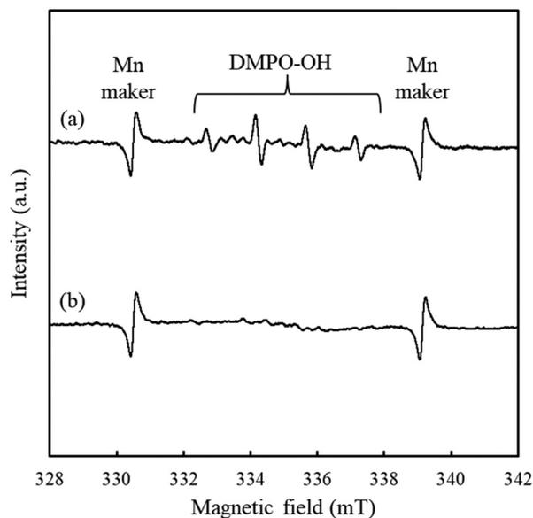
Fig. 8 ESR spectra of (a) DMPO–OH radical observed in an aqueous DMPO solution after immersion of F40, and (b) as-prepared DMPO solution without film immersion.
