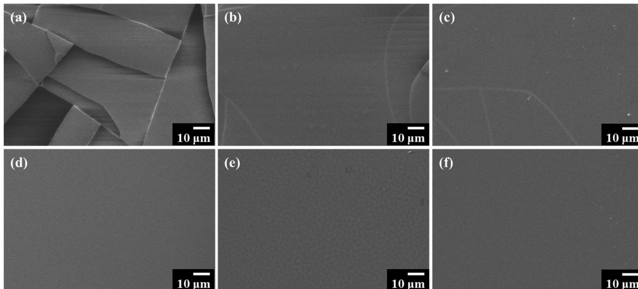
Fig. 2 SEM images of UV-irradiated films: (a) **F35**, (b) **F40**, (c) **F45**, (d) **F50**, (e) **F60**, and (f) **F40H** (obtained by heat treatment of **F40**). All the samples were sputtered with Pt for 20 s to improve surface conductivity before observation.
