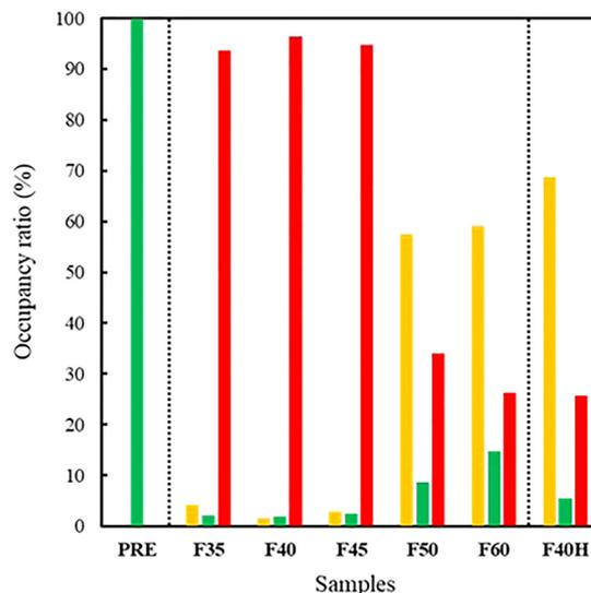
Fig. 5 Occupancy (%) of  $\text{Cu}^+$  (yellow),  $\text{Cu}^{2+}$  (green), and  $\text{Cu}^{3+}$  (red) ions, as analyzed from the Cu  $2p_{3/2}$  peaks in the XPS spectra of UV-irradiated film (FX, X = controlled humidity in the range of 35–60%), and F40H (obtained by heat treatment of F40).
