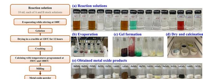
Fig. 1 Schematic illustration of the catalyst synthesis process.
