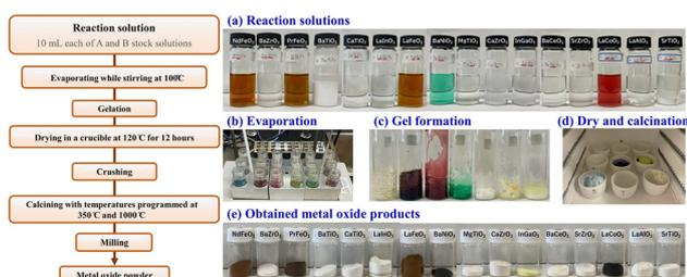
Fig. 1 Schematic illustration of the catalyst synthesis process.
