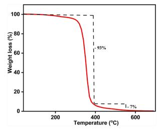
Fig. 3 TGA plot of APBT at a heating rate of 10 °C minute<sup>-1</sup>.
