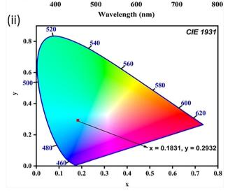
Fig. 7 (i) The prototype LED demo with emission spectrum ( $\lambda_{ex}$ 410 nm); (ii) CIE diagram of its emission.
