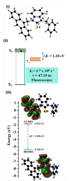
Fig. 6 (i) Optimized geometry of APBT. (ii) The proposed decay scheme of LLCT. (iii) HOMO-LUMO energy gap of APBT.
