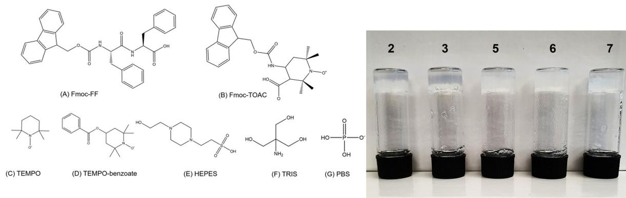
**Fig. 1** Left: Chemical structures of the used materials, (A) Fmoc protected FF dipeptide, (B)–(D) used spin probes: Fmoc-TOAC, TEMPO and TEMPO-benzoate, (E)–(G) buffer molecules: HEPES, TRIS and PBS. Right: Examples of prepared hydrogels (inversion test). Samples are numbered according to Table 1.
