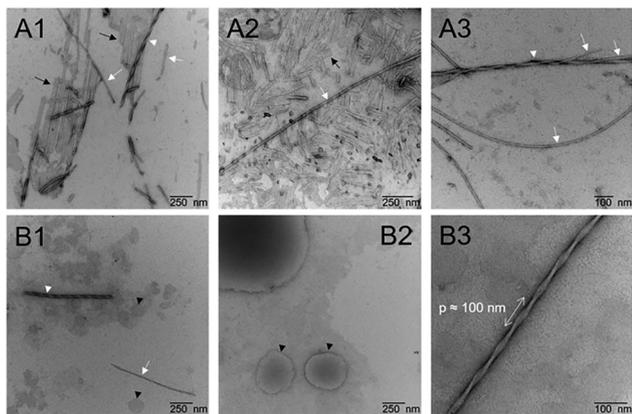
Fig. 3 TEM images of 2 mg mL<sup>-1</sup> Fmoc-FF-Fe hydrogels (A1–3) and Fmoc-FF-Al hydrogels (B1–3) at different magnifications. White arrows point to thin fibers and white arrow heads indicate helical fibers with a pitch ( $p$ ) of around 100 nm. Black arrow heads point to LLPS droplets.
