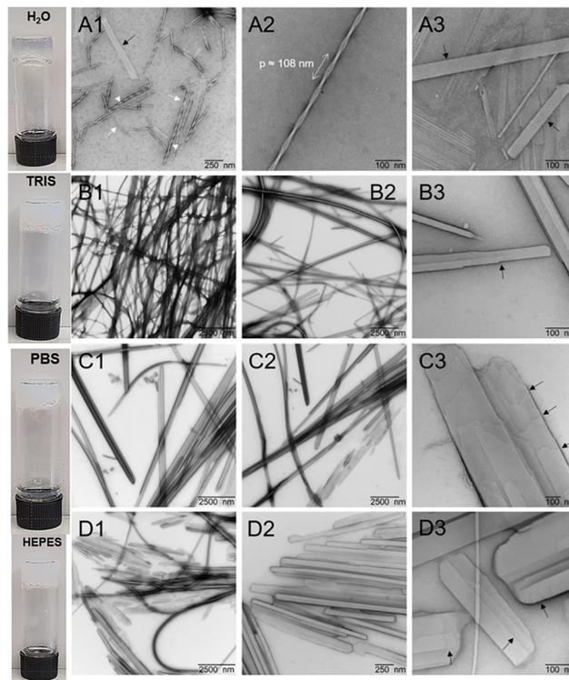
Fig. 2 TEM images of  $2\text{ mg mL}^{-1}$  Fmoc-FF gels in water (A1–3), TRIS (B1–3), PBS (C1–3), and HEPES (D1–3) at different magnifications. White arrows point to thin fibers and white arrow heads indicate helical fibers with a pitch ( $p$ ) of around  $100\text{ nm}$ . Black arrows point to ribbons with terraces. Corresponding invert test tube of each buffered gel is shown on the right side.
