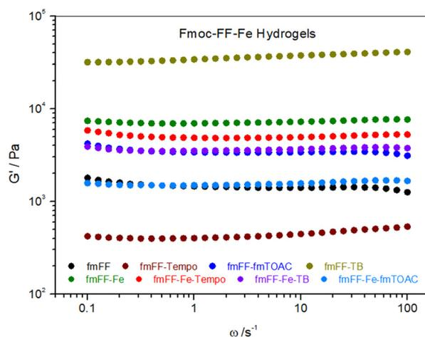
Fig. 7 Frequency-dependent rheological characteristics (storage modulus) of spin probed Fmoc-FF-hydrogels in combinations with  $\text{Fe}^{3+}$  and the three spin probes used in this study. In the figure legend, Fmoc is abbreviated as fm, for the sake of brevity.
