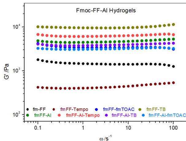
Fig. 6 Frequency-dependent rheological characteristics (storage modulus) of spin probed Fmoc-FF-hydrogels in combinations with  $\text{Al}^{3+}$  and the three spin probes used in this study. In figure legend, Fmoc is abbreviated as fm, for the sake of legend placement.
