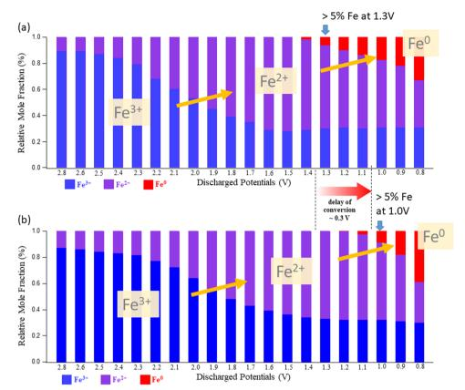
Fig. 4 Linear combination fitting analysis (LCA) for (a) bare FeOF and (b) LiPON-coated FeOF.
