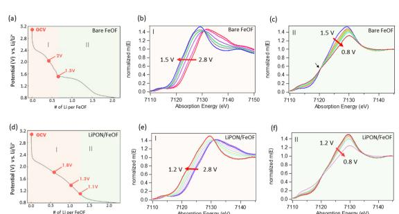
Fig. 2 (a) Discharge profile of bare FeOF; XANES spectra of bare FeOF discharged in (b) region I of 2(a) - OCV ~ 1.5 V; (c) region II (1.5-0.8 V). (d) Discharge profile of LiPON-coated FeOF; XANES spectra of LiPON-coated FeOF discharged in (e) region I of 2(d) –OCV ~1.2 V; (f) region II of 2(d) -1.2-0.8 V
