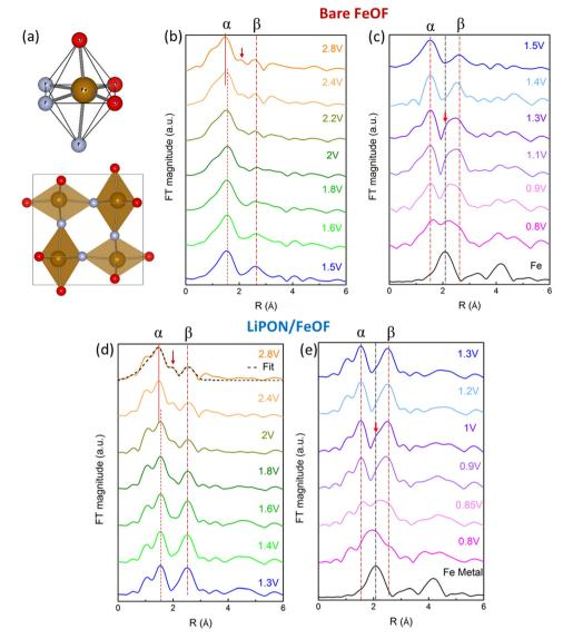
Fig. 3 (a) Crystal structure of FeOF. (Upper) Octahedral site of Fe. (Lower) Unit cell of FeOF with projection along [001], and RDF plots of (b) and (c) bare FeOF and (d) and (e) coated FeOF, where  $\alpha$  indicates the Fe-O scattering path and  $\beta$  corresponds to Fe-Fe scattering of FeOF.
