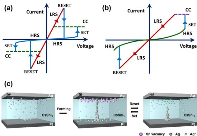
**Fig. 1** (a) Unipolar Switching mode of the resistive switching memory devices. (b) Bipolar Switching mode of the resistive switching memory devices. Reproduced with permission from ref. 59. Copyright 2013, Springer. (c) The ECM process of the resistive switching memory devices. Reproduced with permission from ref. 70. Copyright 2019, American Chemical Society.
