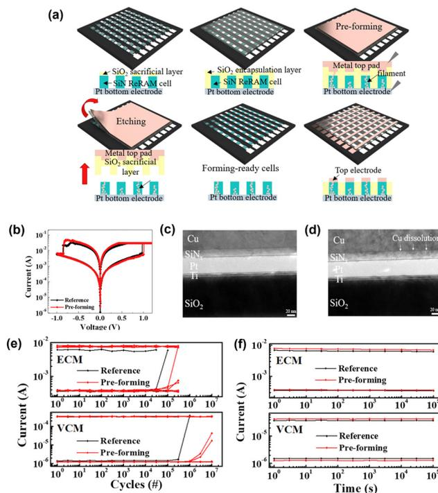
Fig. 4 (a) Process flow of the pre-forming method. (b)  $I$ - $V$  curves of reference and pre-formed devices. (c) TEM images of the devices before the pre-forming process. (d) TEM images of the devices after the pre-forming process. (e) Endurance cycles of reference and pre-formed devices. (f) Retention time of reference and pre-formed devices. Reproduced with permission from ref. 80. Copyright 2020, Elsevier.
