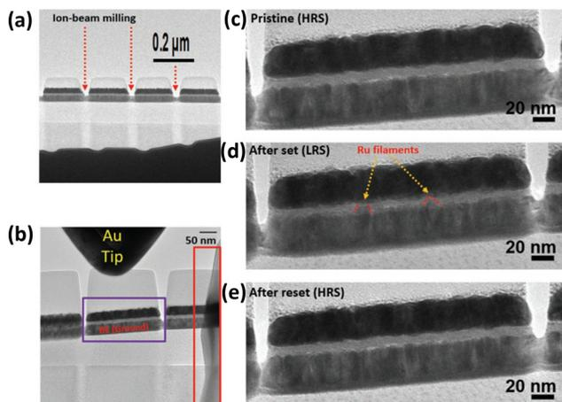
Fig. 7 (a) Bright-field TEM image of the fabricated individual nanopillar-type *in situ* TEM sample, and (b) depiction of the contact formation between the Au tip and the top electrode during bias application. (c)–(e) Cross-sectional *in situ* TEM images of the Pd/Pt (top)/Ta<sub>2</sub>O<sub>5</sub>/Ru (bottom) structured device, illustrating its pristine HRS, LRS, and RESET HRS. Reproduced with permission from ref. 98. Copyright 2020, Wiley.
