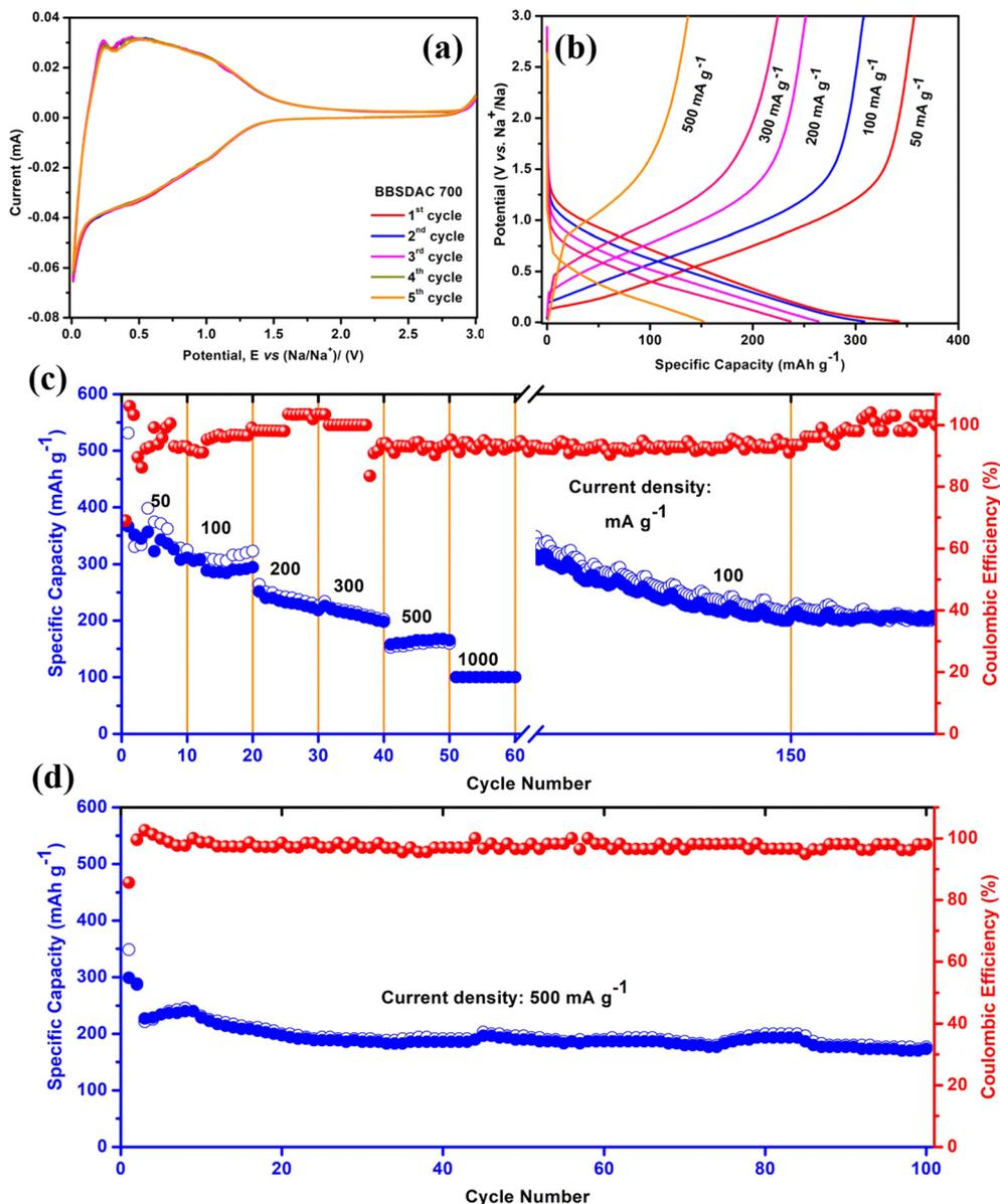
Fig. 2 Electrochemical performance of the half cells. (a) CV curves of the first five cycles at a scan rate of  $0.1 \text{ mV s}^{-1}$ , (b) charge–discharge profiles with different current density, (c) rate capability and coulombic efficiency at different current density and (d) long-term cycling study and coulombic efficiency at  $500 \text{ mA g}^{-1}$  of BBSDAC 700.
