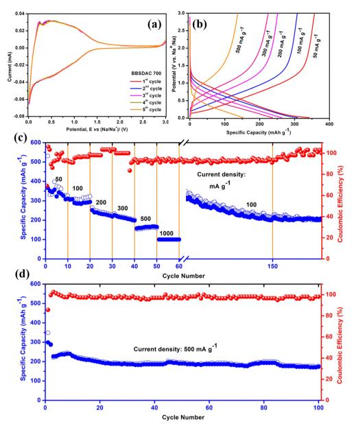
Fig. 2 Electrochemical performance of the half cells. (a) CV curves of the first five cycles at a scan rate of  $0.1 \,\mathrm{mV} \,\mathrm{s}^{-1}$ , (b) charge–discharge profiles with different current density, (c) rate capability and coulombic efficiency at different current density and (d) long-term cycling study and coulombic efficiency at 500 mA  $\,\mathrm{g}^{-1}$  of BBSDAC 700.
