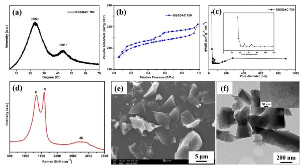
(a) XRD pattern, (b) N<sub>2</sub> adsorption/desorption isotherm, (c) pore distribution, (d) Raman spectrum, (e) SEM and (f) TEM for the BBSDAC 700.
