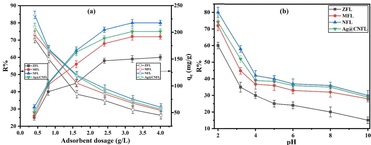
Fig. 3 Adsorbent dosage (a) and pH (b) effects for 2,4-D adsorption onto ZFL, MFL, NFL, and Ag@CNFL at 300 mg L<sup>-1</sup> 2,4-D concentration for 20 h of shaking time at 23 °C.
