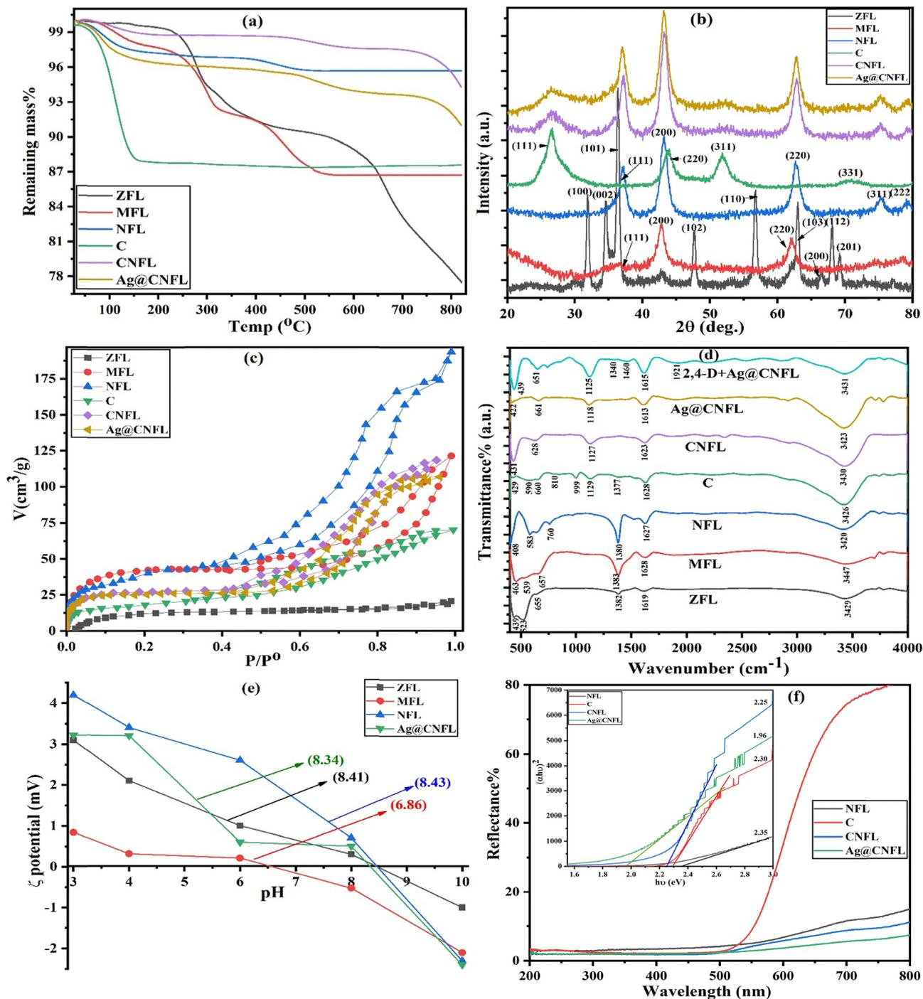
Fig. 1 TGA (a), XRD (b), N<sub>2</sub> adsorption (c), and ATR-FTIR (d) of all the samples, zeta potential (e) of adsorbents, UV-vis DRS (inset: band gap energy values) (f) curves of the catalysts, and, the ATR-FTIR curve of Ag@CNFL after 2,4-D adsorption.
