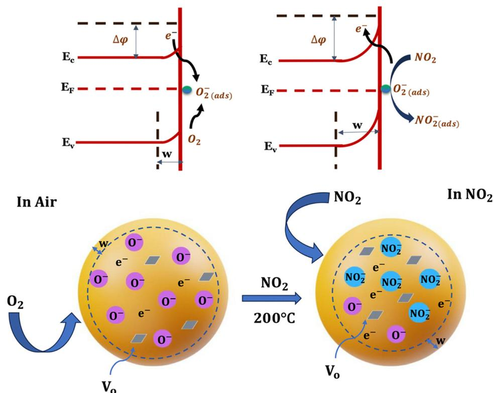
Fig. 12 Mechanism of gas sensing and band bending in EBI Cr- $WO_3$  film.
