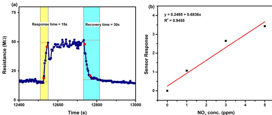
Fig. 10 (a) Response and recovery kinetics of sample C at 5 ppm  $\text{NO}_2$  and 200 °C. (b) Linear regression graph illustrating the sensor response as a function of  $\text{NO}_2$  concentration for sample C at 200 °C.
