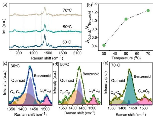
Fig. 5 (a) Raman spectra of PEDOT:PSS films at various temperatures between 30 °C and 70 °C after exposure to NIR light. (b) Quinoid and benzenoid structural transition trend. (c)–(e) The deconvoluted Raman spectra at various temperatures when MPS is exposed to NIR light.
