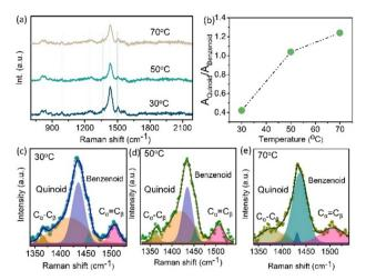
Fig. 5 (a) Raman spectra of PEDOT:PSS films at various temperatures between 30  $^{\circ}$ C and 70  $^{\circ}$ C after exposure to NIR light. (b) Quinoid and benzenoid structural transition trend. (c)–(e) The deconvoluted Raman spectra at various temperatures when MPS is exposed to NIR light.
