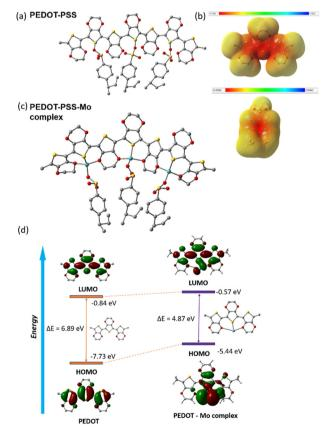
**Fig. 6** (a) Gauss structure of PEDOT:PSS. (b) Molecular electrostatic potential (MEP) of PEDOT (left) and PSS (right). (c) Gauss structure of the PEDOT-PSS with Mo complex. (d) Energy optimized structures of PEDOT and the PEDOT with Mo complex.
