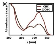
Fig. 5 Absorbance spectra for coumarin containing micelles used to validate the crosslinking associated with micelle persistence at each processing stage from (a) solution, (b) to polymer films, and (c) after use as templates for nanomaterials. The spectra for non-crosslinked and crosslinked samples are easily distinguished in each case. Data is normalized at 210 nm.
