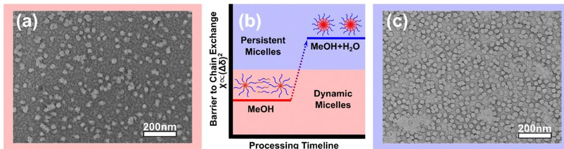
Fig. 2 (a) TEM image of X-OBC–MeOH showing a mixture of micelles and unimers (“fingerprint” background). (b) Water was added to the processing solution to reduce the critical micelle concentration and suppress unimers (increasing  $\chi N$ ). (c) TEM of X-OBC–MeOH–H<sub>2</sub>O showing micelles alone. TEM samples were stained with UrAc so that the PPEGMA appears dark.
