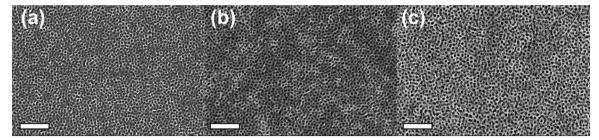
SEM images of X-OBC-THF series with material: template ratio: (a) 0.6, (b) 1.0, (c) 1.4. Scale bars are 200 nm.
