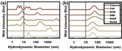
Fig. 4 (a) DLS plots of OBC directly dispersed in various solvents with many conditions releasing substantial unimer fractions (<10 nm, dashed line) as compared to (b) DLS of X-OBC micelles which persisted as micelles under all conditions tested without detectable unimer release.
