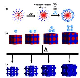
Overview showing the preparation and use of X-OBC templates. (a) OBC micelles are irradiated with UV light to induce crosslinking where subsequent addition of nanoparticles selectively associate with the hydrophilic corona. (b) With persistent micelle templates, the resulting pore size is constant with such material additions which enable tailored wall thickness. (c) Subsequent calcination removes the polymer and results in pores.
