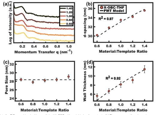
Fig. 8 (a) SAXS data for TiO<sub>2</sub> combined with crosslinked X-OBC with variable loading extents. (b) The corresponding d-spacings were consistent with the PMT model. Direct SEM measurements of (c) pore size and (d) wall thickness was also both consistent with the PMT model. Samples were processed from THF and the SAXS data were shifted vertically for clarity.
