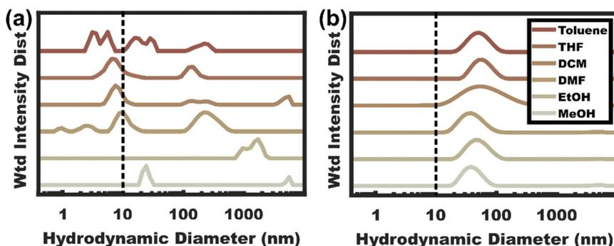
Fig. 4 (a) DLS plots of OBC directly dispersed in various solvents with many conditions releasing substantial unimer fractions ( $< 10$  nm, dashed line) as compared to (b) DLS of X-OBC micelles which persisted as micelles under all conditions tested without detectable unimer release.
