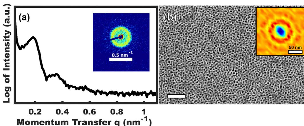
Fig. 6 Representative dataset for sample X-OBC-THF (a) SAXS and (b) SEM. The integrated SAXS pattern is shown with the 2D pattern inset. The color scale corresponds to the log-scale of the X-ray intensity. The SEM image has light areas that correspond to the  $\text{TiO}_2$  whereas the dark areas correspond to pores produced by removing the X-OBC template. The inset in (b) is the 2D spatial distribution function derived from the SEM image. Scale bar is 200 nm.
