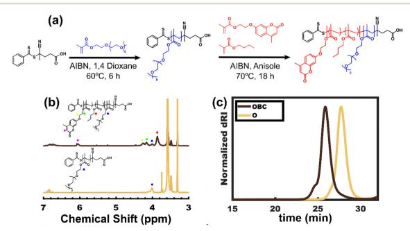
Fig. 1 (a) Synthesis scheme for O homopolymer (PPEGMA) followed by chain extensions of BC using RAFT polymerization. Both O and OBC were characterized by (b) <sup>1</sup>H-NMR spectra and (c) GPC analysis.
