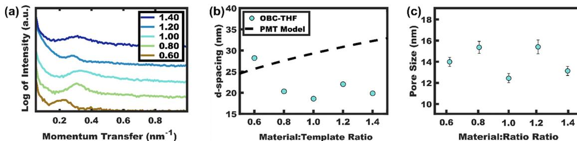
Fig. 7 (a) SAXS data for  $\text{TiO}_2$  combined with uncrosslinked OBC with variable material:template loading. (b) The corresponding  $d$ -spacing and (c) average pore sizes were similarly sporadic, suggesting dynamic micelles that were inconsistent with the expectations for persistent micelles. Samples were processed from THF and the SAXS data were shifted vertically for clarity.
