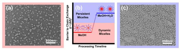
Fig. 2 (a) TEM image of X-OBC-MeOH showing a mixture of micelles and unimers ("fingerprint" background). (b) Water was added to the processing solution to reduce the critical micelle concentration and suppress unimers (increasing  $\chi N$ ). (c) TEM of X-OBC-MeOH-H<sub>2</sub>O showing micelles alone. TEM samples were stained with UrAc so that the PPEGMA appears dark.
