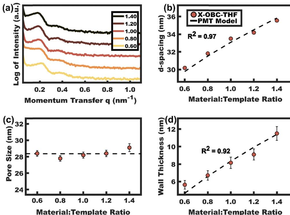
Fig. 8 (a) SAXS data for  $\text{TiO}_2$  combined with crosslinked X-OBC with variable loading extents. (b) The corresponding  $d$ -spacings were consistent with the PMT model. Direct SEM measurements of (c) pore size and (d) wall thickness was also both consistent with the PMT model. Samples were processed from THF and the SAXS data were shifted vertically for clarity.
