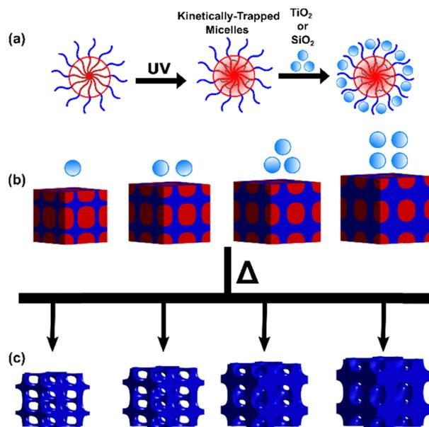
**Scheme 1** Overview showing the preparation and use of X-OBC templates. (a) OBC micelles are irradiated with UV light to induce crosslinking where subsequent addition of nanoparticles selectively associate with the hydrophilic corona. (b) With persistent micelle templates, the resulting pore size is constant with such material additions which enable tailored wall thickness. (c) Subsequent calcination removes the polymer and results in pores.
