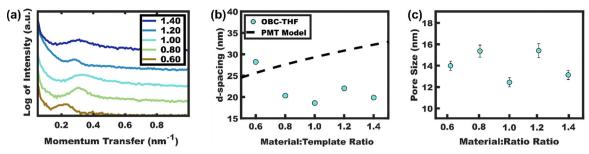
Fig. 7 (a) SAXS data for TiO<sub>2</sub> combined with uncrosslinked OBC with variable material:template loading. (b) The corresponding d-spacing and (c) average pore sizes were similarly sporadic, suggesting dynamic micelles that were inconsistent with the expectations for persistent micelles. Samples were processed from THF and the SAXS data were shifted vertically for clarity.
