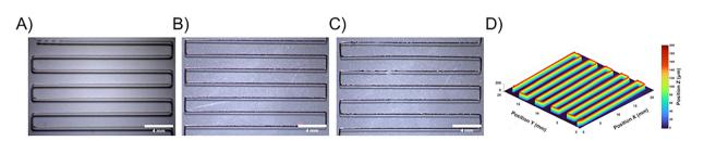
Fig. 6 Stereomicroscopy images of (A) PCL, (B) PCL-P3HT-1 and (C) PCL-P3HT-4 digital snakes printed using the 120 °C\_700 kPa\_4 mm s<sup>-1</sup> parameters. Scale bars are 4 mm. (D) Profilometry 3D mapping of the sample presented in (A).
