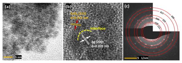
Fig. 4 (a) HRTEM image, (b) interplanar d-spacings, and (c) SAED pattern of Ag/CeO $_2$  nanocomposites.
