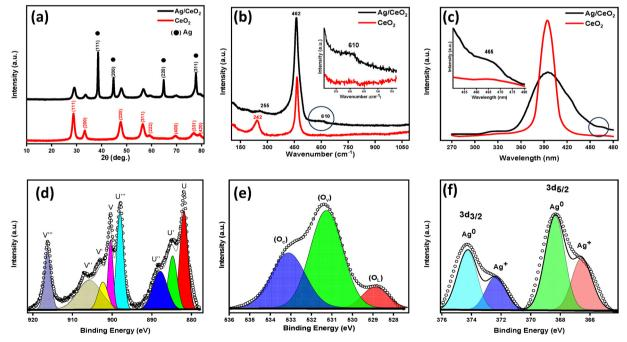
Fig. 1 (a) XRD patterns, (b) Raman spectra, and (c) PL spectra of CeO<sub>2</sub> and Ag/CeO<sub>2</sub> nanocomposites and the XPS spectra and (d) deconvoluted spectra of Ce 3d, (e) O 1s, and (f) Ag 3d for Ag/CeO2 nanocomposites.
