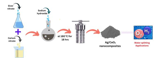
Scheme 1 Preparation of Ag/CeO<sub>2</sub> nanocomposites by a solvothermal method and their application in water splitting
