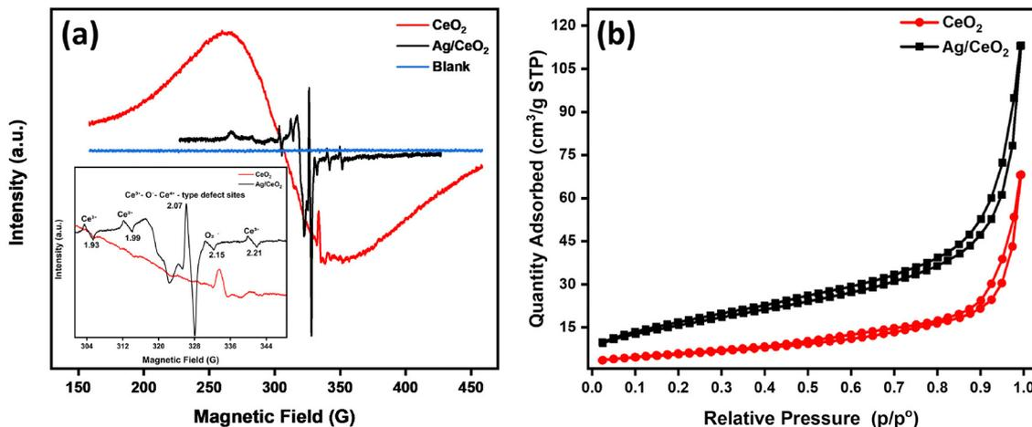
Fig. 2 (a) EPR profiles measured (inset: the calculated  $g$  factor value) at room temperature and (b) BET analysis for  $\text{CeO}_2$  and  $\text{Ag/CeO}_2$  nanocomposites.
