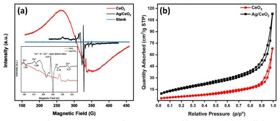
Fig. 2 (a) EPR profiles measured (inset: the calculated g factor value) at room temperature and (b) BET analysis for CeO<sub>2</sub> and Ag/CeO<sub>2</sub> nanocomposites.
