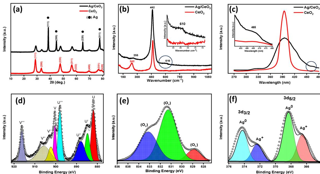
Fig. 1 (a) XRD patterns, (b) Raman spectra, and (c) PL spectra of CeO<sub>2</sub> and Ag/CeO<sub>2</sub> nanocomposites and the XPS spectra and (d) deconvoluted spectra of Ce 3d, (e) O 1s, and (f) Ag 3d for Ag/CeO<sub>2</sub> nanocomposites.
