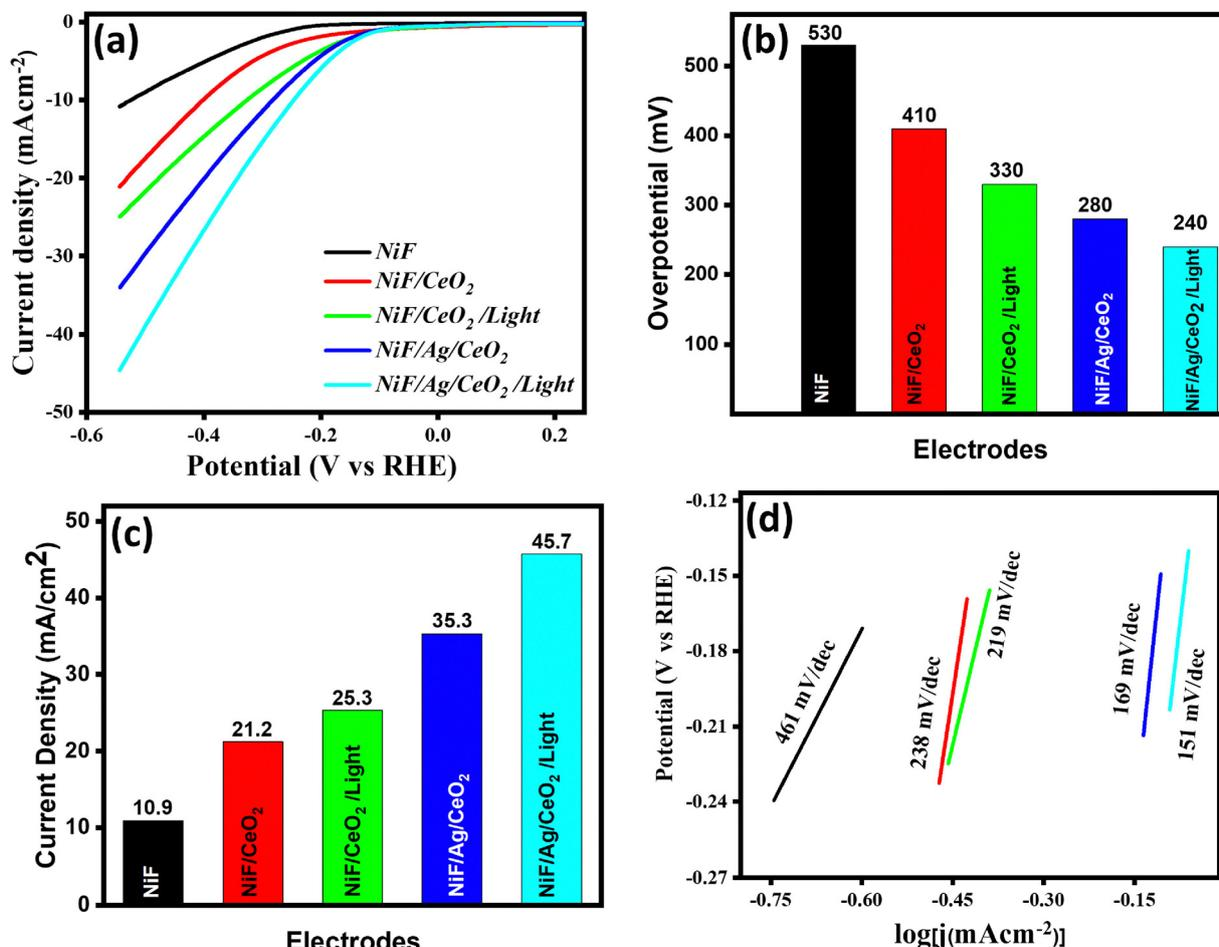
Fig. 6 (a) LSV curves, (b) overpotential (vs. RHE) at a current density of 10 mA cm<sup>-2</sup>, (c) current density at a potential of -0.54 V, and (d) the Tafel slope for the HER of NiF, NiF/CeO<sub>2</sub>, NiF/CeO<sub>2</sub>/Light, NiF/Ag/CeO<sub>2</sub>, and NiF/Ag/CeO<sub>2</sub>/Light.
