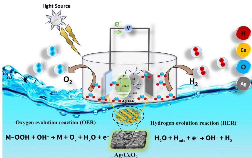
**Fig. 7** Mechanism of the electrocatalytic water splitting.
