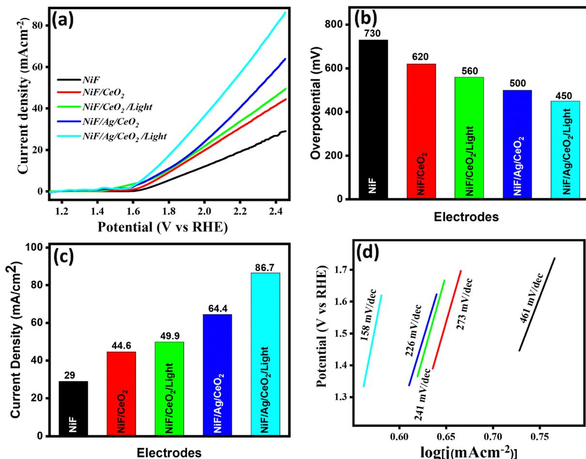
Fig. 5 (a) LSV curves, (b) overpotential (vs. RHE) at a current density of 10 mA cm<sup>-2</sup>, (c) current density at a potential of 2.4 V, and (d) the Tafel slope for the OER of NiF, NiF/CeO<sub>2</sub>, NiF/CeO<sub>2</sub>/Light, NiF/Ag/CeO<sub>2</sub>, and NiF/Ag/CeO<sub>2</sub>/Light.
