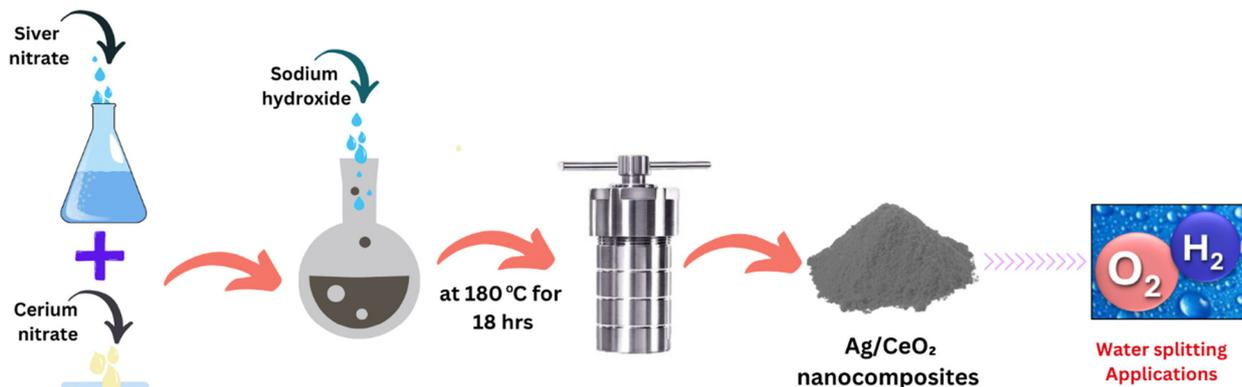
Scheme 1 Preparation of Ag/CeO<sub>2</sub> nanocomposites by a solvothermal method and their application in water splitting.
