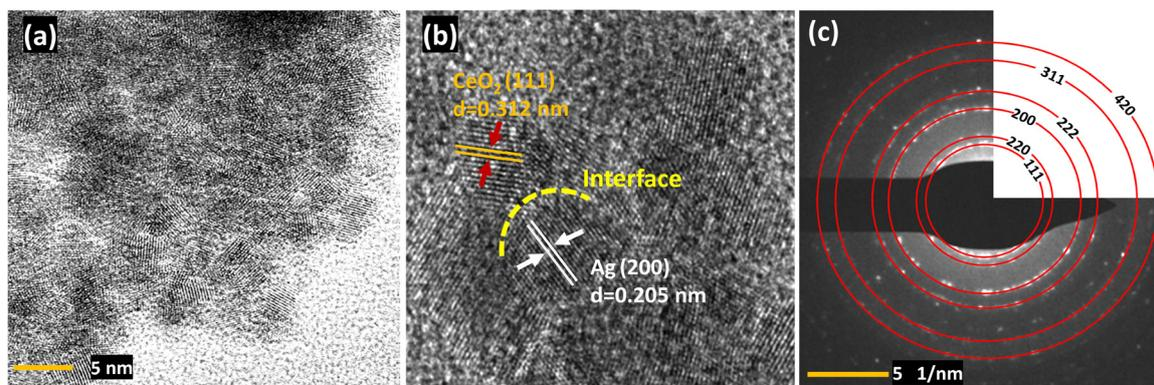
Fig. 4 (a) HRTEM image, (b) interplanar *d*-spacings, and (c) SAED pattern of Ag/CeO<sub>2</sub> nanocomposites.
