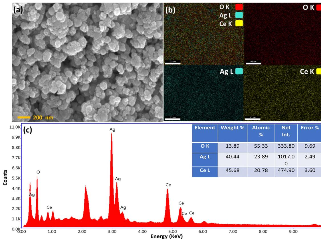
Fig. 3 (a) High-magnification FESEM images, (b) EDX elemental mapping, and (c) EDX spectrum of Ag/CeO<sub>2</sub> (inset: atomic and weight percentages of elements present in Ag/CeO<sub>2</sub> nanocomposites).
