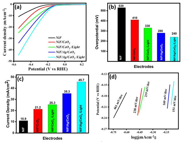
Fig. 6 (a) LSV curves, (b) overpotential (vs. RHE) at a current density of 10 mA cm $^{-2}$ , (c) current density at a potential of -0.54 V, and (d) the Tafel slope for the HER of NiF, NiF/CeO<sub>2</sub>/Light, NiF/Ag/CeO<sub>2</sub>, and NiF/Ag/CeO<sub>2</sub>/Light.
