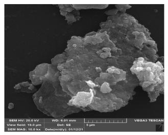
Fig. 4 SEM image of the Gu-GO/Fe<sub>3</sub>O<sub>4</sub> nanocomposite.
