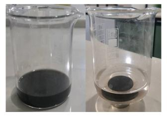
Fig. 7 Magnetic separation ability of the Gu-GO/Fe<sub>3</sub>O<sub>4</sub> nanocomposite
