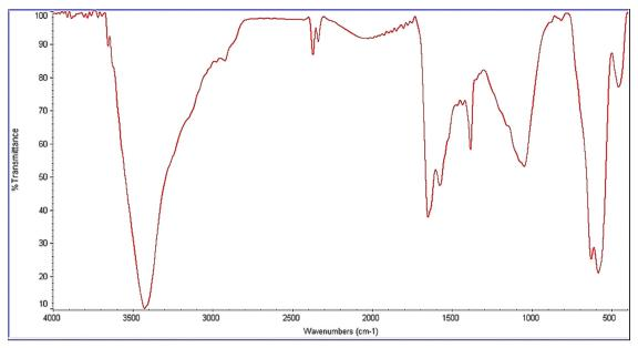
Fig. 11 FT-IR spectrum of the recovered Gu-GO/Fe<sub>3</sub>O<sub>4</sub> catalyst.
