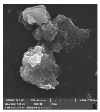
Fig. 10 The SEM image of the recovered Gu-GO/Fe<sub>3</sub>O<sub>4</sub> catalyst.
