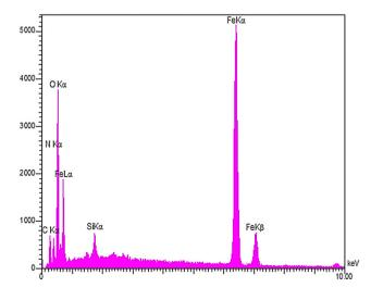
Fig. 2 EDX analysis of the Gu-GO/Fe<sub>3</sub>O<sub>4</sub> nanocomposite.
