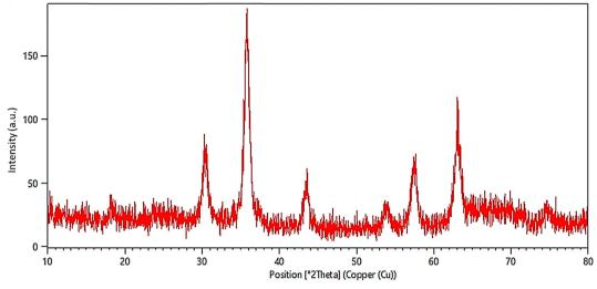
Fig. 5 XRD pattern of the Gu-GO/Fe<sub>3</sub>O<sub>4</sub> nanocomposite.
