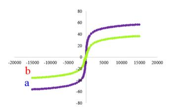
Fia. 6 VSM diagrams of the  $Fe_3O_4$ Gu-GO/Fe₃O₄ (a) (b) and nanocomposite.
