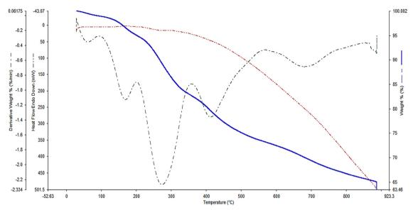
Fig. 8 TGA analysis of the Gu-GO/Fe<sub>3</sub>O<sub>4</sub> nanocomposite.
