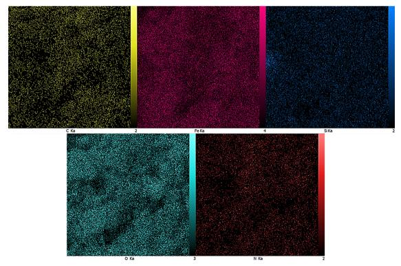
Fig. 3 EDX mapping analysis of the Gu-GO/Fe<sub>3</sub>O<sub>4</sub> nanocomposite.
