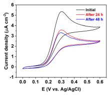
Fig. 3 CVs of the electrode modified with GOx immobilized in the hydrogel towards 6 mM glucose in 0.1 M pH 7 PBS. Scan rate: 5 mV  $\rm s^{-1}$ Storage condition: 4 °C
