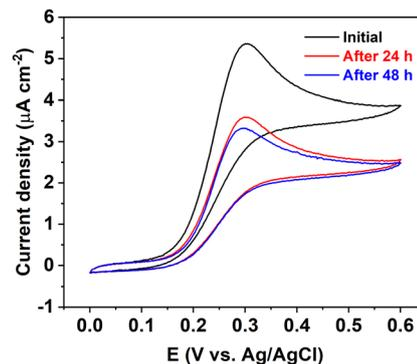
Fig. 3 CVs of the electrode modified with GOx immobilized in the hydrogel towards 6 mM glucose in 0.1 M pH 7 PBS. Scan rate: 5 mV s<sup>-1</sup>. Storage condition: 4 °C.
