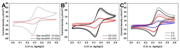
Fig. 2 CVs of the UV cured hydrogel using (A) Bzp-dex with two different MWs, (B) CD-dex with two different DSs and (C) different molecular ratios of introduced Fc to CD-dex. Solution: 0.1 M pH 7 PBS. Scan rate: 100 mV s<sup>-1</sup>
