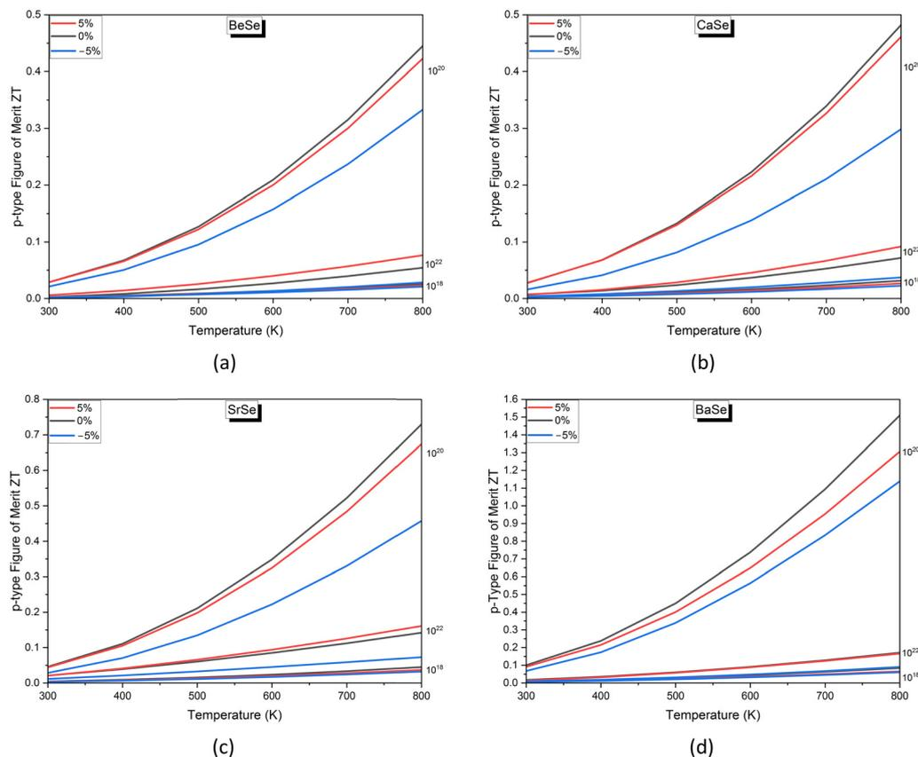
Fig. 12 Temperature-dependent figures of merit ( $ZT$ ) for P-type AEMSe at different strain levels ( $-5\%$ ,  $0\%$ , and  $+5\%$ ) and doping concentrations of  $10^{18}$ ,  $10^{20}$  and  $10^{22} \text{ cm}^{-3}$ .
