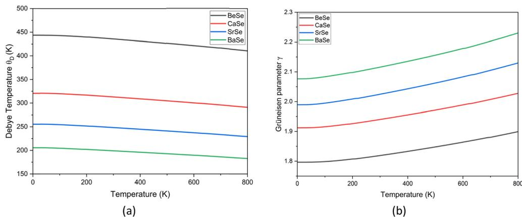
Fig. 4 Temperature-dependent properties of the AEMSe compounds: (a) Debye temperature in Kelvin, and (b) Grüneisen parameter.
