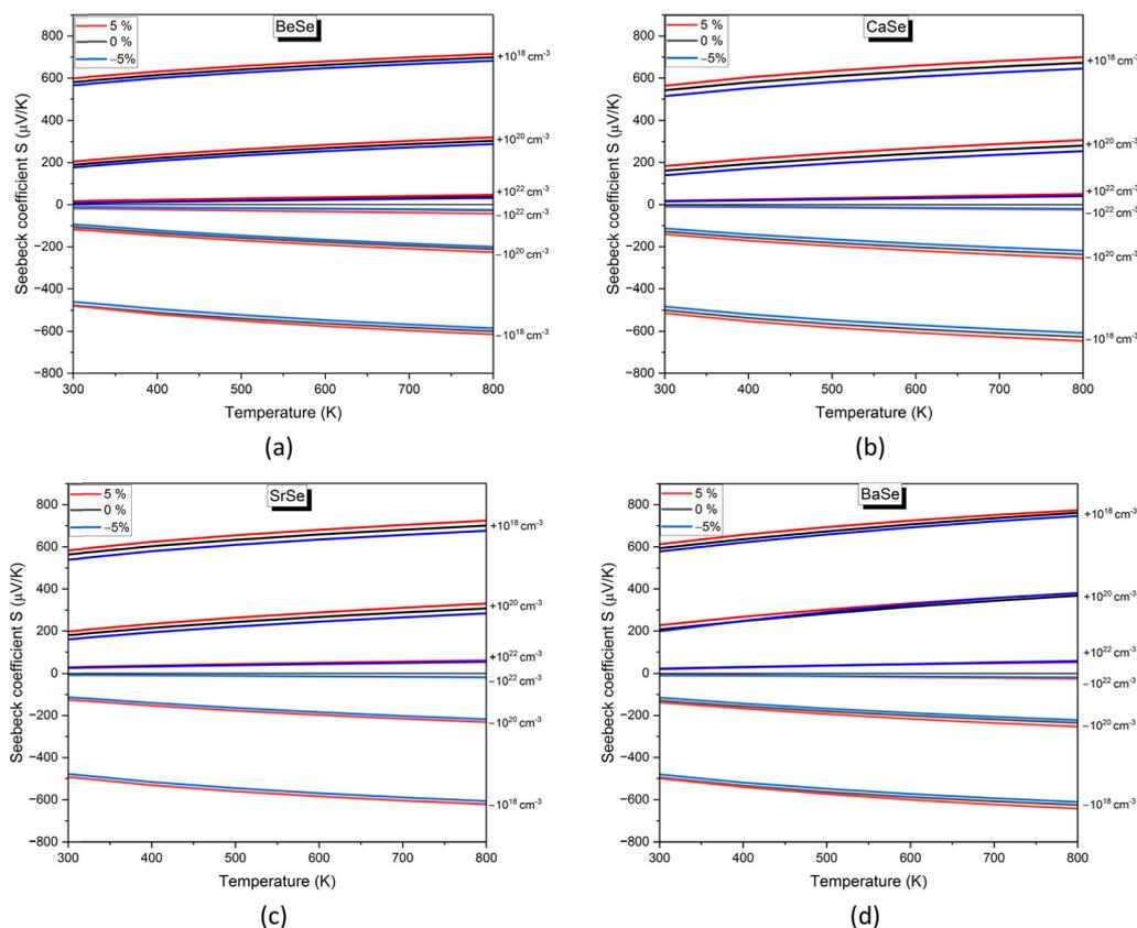
**Fig. 6** Variation of the Seebeck coefficient with temperature for AEMSe compounds under compressive strain (−5%), unstrained (0%), and tensile strain (+5%). The results are shown for doping concentrations of  $10^{18}$ ,  $10^{20}$ , and  $10^{22} \text{ cm}^{-3}$ , considering both positive (P-type) and negative (N-type) charge carriers.
