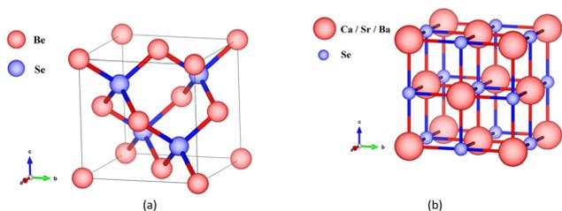
Fig. 1 Crystal structures of AEMSe compounds: (a) BeSe adopting the ZnS phase with an FCC structure. (b) CaSe, SrSe, and BaSe naturally adopting the NaCl phase with an FCC structure.<sup>28</sup>
