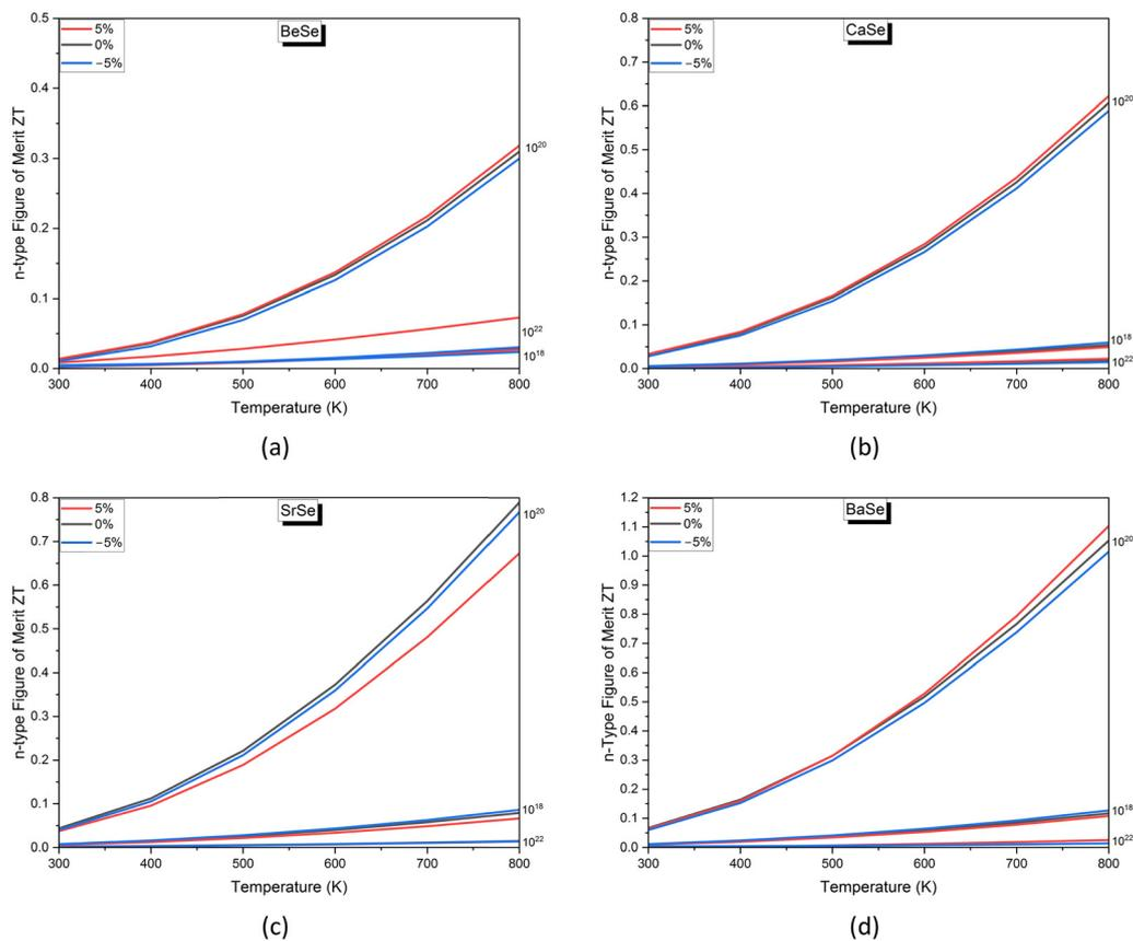
Fig. 11 Temperature-dependent figure of merit ( $ZT$ ) for N-type AEMSe at different strain levels ( $-5\%$ ,  $0\%$ , and  $+5\%$ ) and doping concentrations of  $10^{18}$ ,  $10^{20}$  and  $10^{22} \text{ cm}^{-3}$ .
