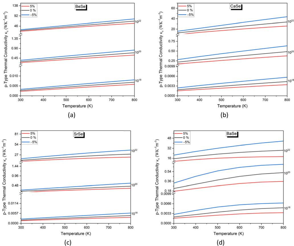
Fig. 10 Variation of electronic thermal conductivity with temperature for the AEMSe under compressive strain (−5%), unstrained conditions (0%), and tensile strain (+5%). Results are presented for P-type doping concentrations of  $10^{18}$ ,  $10^{20}$ , and  $10^{22}$   $\text{cm}^{-3}$ , showing the influence of strain and doping on electronic thermal conductivity.
