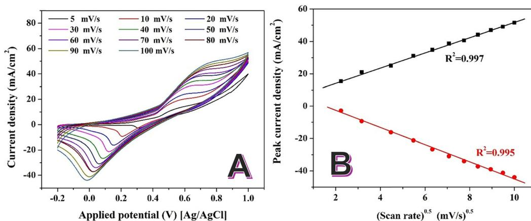
Fig. 8 Cyclic voltammetry curves of the Ni–NiCr–CNFs (15 wt% sample) electrode at different scan rates (5–100  $\text{mV s}^{-1}$ ) in 0.05 M glycerol with 1.0 M KOH as the supporting electrolyte; (A), and the relationship between the anodic and cathodic peak current densities and the square root of the scan rate; (B).
