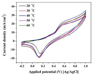
Fig. 9 Effect of reaction temperature on the electrocatalytic activity of the Ni-NiCr-CNFs nanofiber electrode using 0.05 M glycerol solution at 50 mV s<sup>-1</sup> scan rate.
