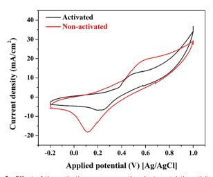
Fig. 6 Effect of the activation process on the electrocatalytic activity of the proposed NiCr-CNFs (15 wt% sample) at 0.05 M glycerol in 1.0 M KOH, scan rate 50 mV s<sup>-1</sup>.
