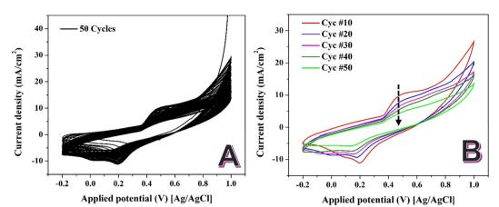
Fig. 4 Sweeping of the prepared NiCr NPs-incorporated carbon nanofibers in 1.0 M KOH at scan rate of 50 mV s<sup>-1</sup> at 25 °C for 50 successive cycles; (A) and selected cycles; (B)
