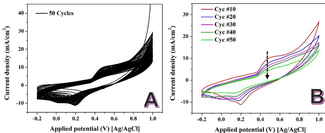
Fig. 4 Sweeping of the prepared NiCr NPs-incorporated carbon nanofibers in 1.0 M KOH at scan rate of  $50 \text{ mV s}^{-1}$  at  $25^\circ \text{C}$  for 50 successive cycles; (A) and selected cycles; (B).
