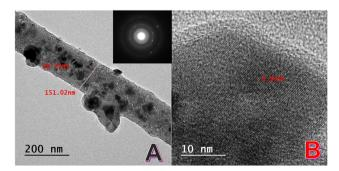
Fig. 3 Normal TEM image; (A) and HR-TEM image; (B) for the prepared NiCr NPs-incorporated CNFs from electrospun solution containing 15 wt% CrAc and calcined at 850 °C. The inset displays SAED pattern for the crystalline nanoparticles.
