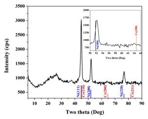
Fig. 1 XRD pattern for the prepared Ni-NiCr NPs-incorporated CNFs from electrospun solution containing 15 wt% CrAc and calcined at 850  $^{\circ}\text{C}$
