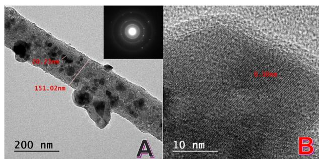
Fig. 3 Normal TEM image; (A) and HR-TEM image; (B) for the prepared NiCr NPs-incorporated CNFs from electrospun solution containing 15 wt% CrAc and calcined at  $850^\circ\text{C}$ . The inset displays SAED pattern for the crystalline nanoparticles.
