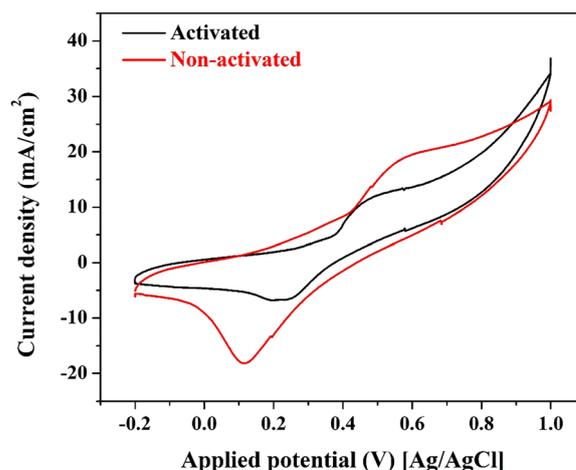
Fig. 6 Effect of the activation process on the electrocatalytic activity of the proposed NiCr–CNFs (15 wt% sample) at  $0.05 \text{ M}$  glycerol in  $1.0 \text{ M KOH}$ , scan rate  $50 \text{ mV s}^{-1}$ .
