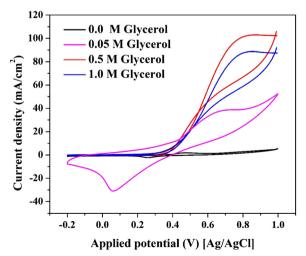
Fig. 5 Electrooxidation of glycerol using the prepared Ni-NiCr NPsincorporated CNFs (15 wt% sample) at different glycerol concentration in 1.0 M KOH solution at 50 mV s $^{-1}$  scan rate and 25 °C.
