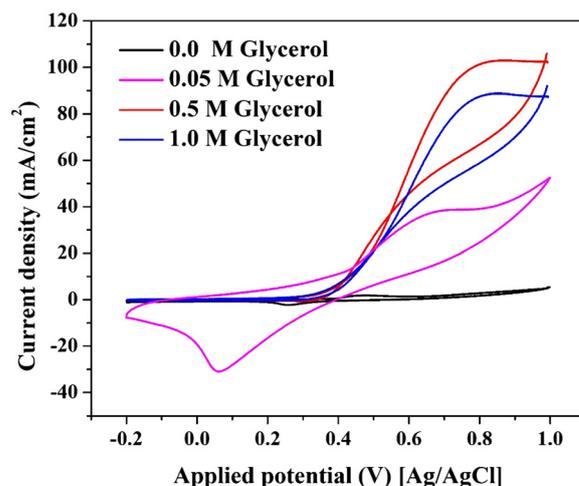
Fig. 5 Electrooxidation of glycerol using the prepared Ni-NiCr NPs-incorporated CNFs (15 wt% sample) at different glycerol concentration in 1.0 M KOH solution at  $50 \text{ mV s}^{-1}$  scan rate and  $25^\circ \text{C}$ .
