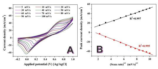
Fig. 8 Cyclic voltammetry curves of the Ni–NiCr-CNFs (15 wt% sample) electrode at different scan rates (5–100 mV s<sup>-1</sup>) in 0.05 M glycerol with 1.0 M KOH as the supporting electrolyte; (A), and the relationship between the anodic and cathodic peak current densities and the square root of the scan rate; (B).
